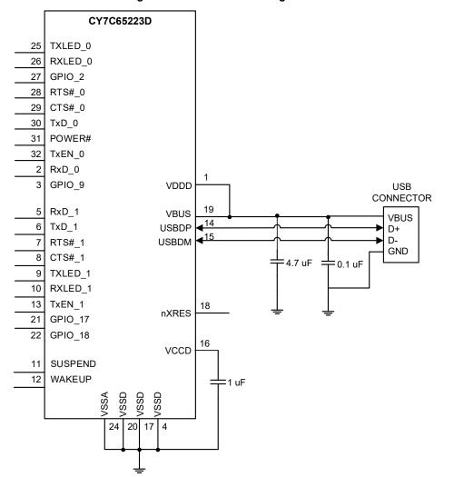
Figure 3. Bus-Powered Configuration
