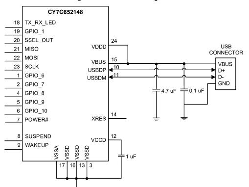
Figure 5. Bus-Powered Configuration
