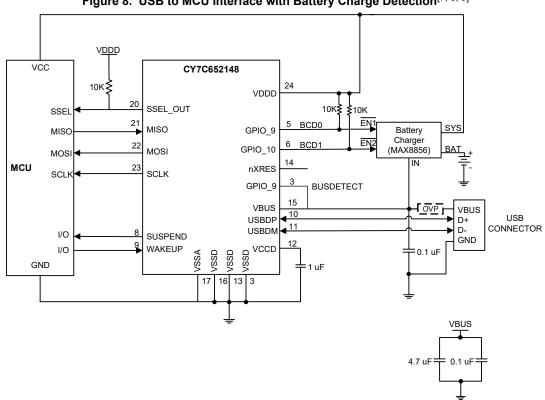
Figure 8. USB to MCU Interface with Battery Charge Detection<sup>[7, 8, 9]</sup>
