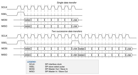
The following figure illustrates a single 8-bit data transfer and two successive 8-bit data transfers. The SSEL pulse coincides with the first data bit.
