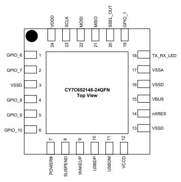
Figure 4. 24-pin QFN Pinout
