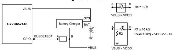
When the VBUS and VDDD are at the same voltage potential, the VBUS can be connected to the GPIO using a series resistor (Rs). This is shown in the following figure. If there is a charger failure and the VBUS becomes 9 V, then the 10-k $\Omega$  resistor plays two roles. It reduces the amount of current flowing into the forward-biased diodes in the GPIO, and it reduces the voltage seen on the pad.
