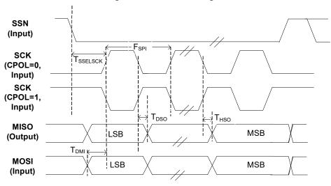
Figure 3. SPI Slave Timing
