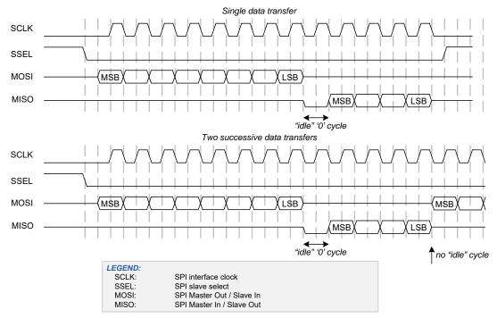
**Note** The above figure defines MISO and MOSI as undefined when the lines are considered idle (not carrying valid information). It will drive the outgoing line values to '0' during idle time (to satisfy the requirements of specific master devices (NXP LPC17xx) and specific slave devices (Microchip EEPROM).
