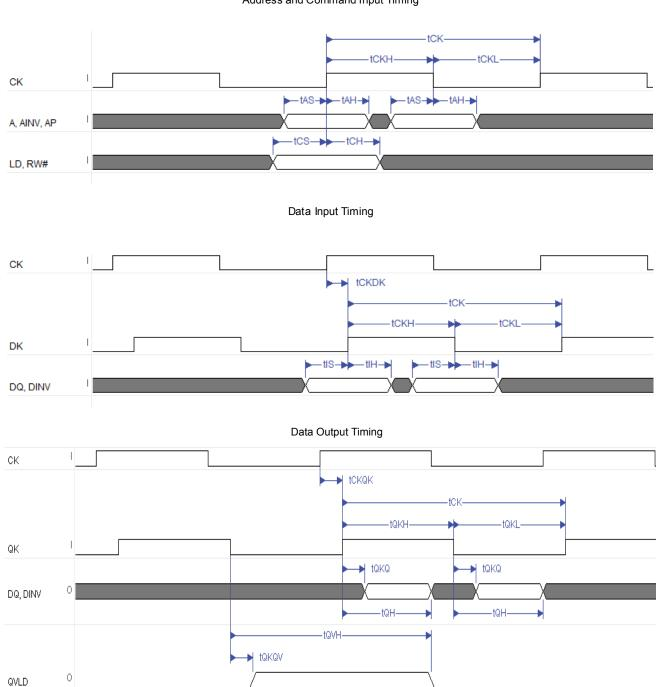
Address and Command Input Timing
