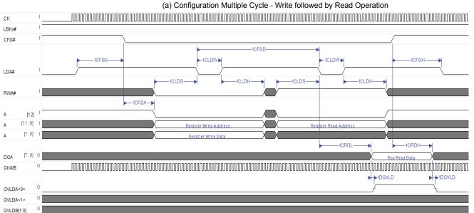
Figure 14. Configuration Write and Read Timing Waveform
