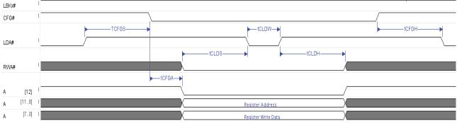
Note: It is recommended to keep CFG# asserted during the configuration write or read operation
