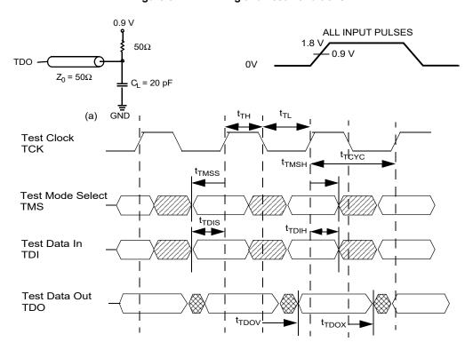
Note 17. Test conditions are specified using the load in TAP AC Test Conditions.  $t_R/t_F$  = 1 ns.
