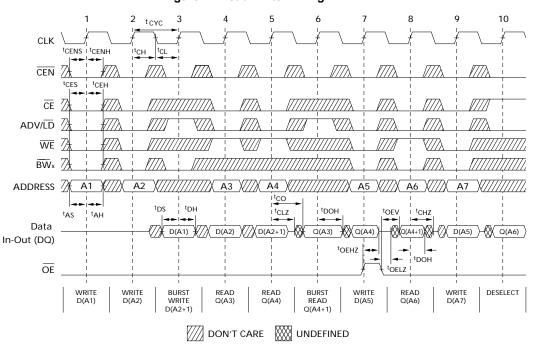
Figure 5. NOP, STALL and DESELECT Cycles [25, 26, 28]
