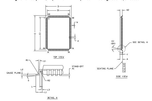
Figure 10. 100-pin TQFP (14 × 20 × 1.4 mm) A100RA Package Outline, 51-85050
