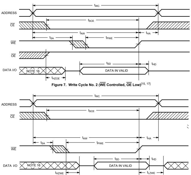
Figure 6. Write Cycle No. 1 (WE Controlled, OE High During Write)<sup>[14, 15]</sup>
