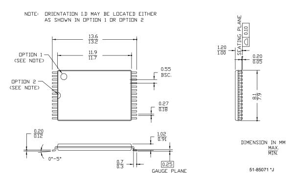
Figure 12. 28-pin TSOP I (8 × 13.4 × 1.2 mm) Z28 (Standard) Package Outline, 51-85071
