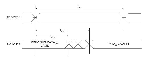
Figure 9. Read Cycle No. 1 of CY62167GE (Address Transition Controlled)  $^{[29,\ 30]}$
