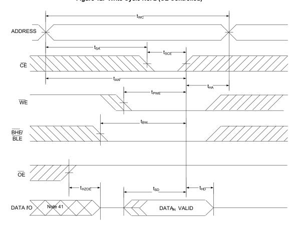
Figure 12. Write Cycle No. 2 (CE Controlled) [38, 39, 40]
