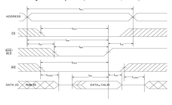
Figure 14. Write Cycle No. 5 (WE Controlled) [42, 43, 44]
