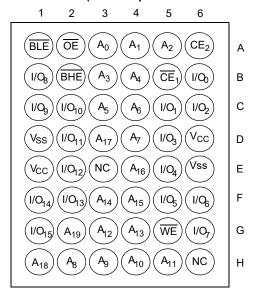
Figure 2. 48-pin TSOP I Pinout (Dual Chip Enable without ERR) - CY62167G [3, 4]
