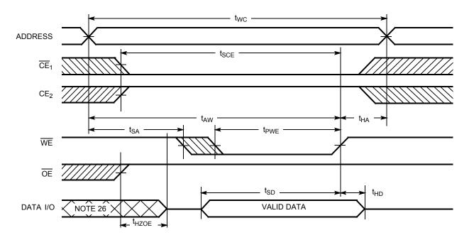
Figure 7. Write Cycle No. 2 ( $\overline{\text{CE}}_1$  or  $\text{CE}_2$  Controlled)  $^{[23,\ 24,\ 25]}$
