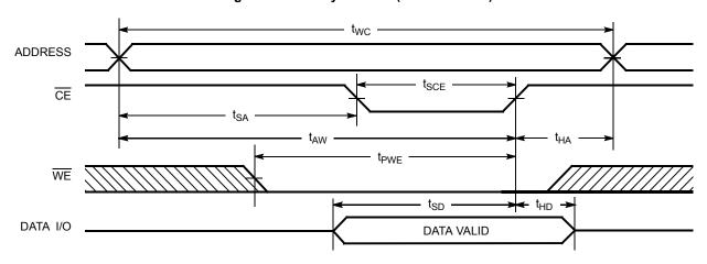
Figure 8. Write Cycle No. 3 (WE Controlled, OE LOW) [27, 28]
