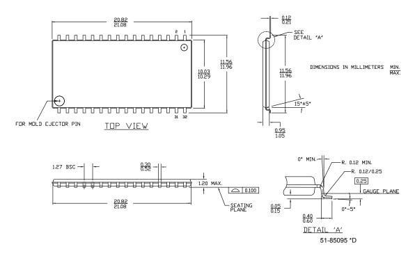
Figure 10. 32-pin SOIC (450 Mils) S32.45/SZ32.45 Package Outline, 51-85081
