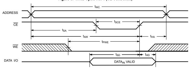
Figure 7. Write Cycle No. 2 (WE Controlled) [27]
