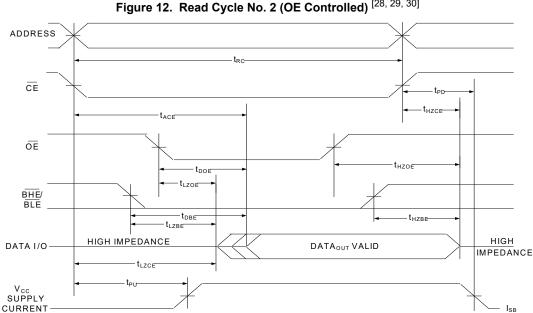
Figure 12. Read Cycle No. 2 (OE Controlled) [28, 29, 30]
