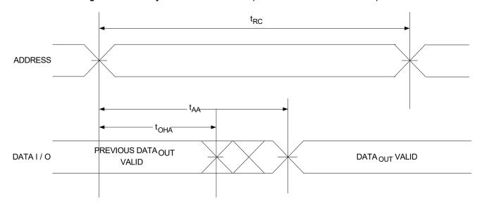
Figure 11. Read Cycle No. 1 of CY62147GE (Address Transition Controlled) [26, 27]
