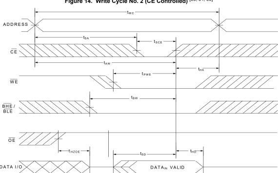
Figure 14. Write Cycle No. 2 (CE Controlled) [33, 34, 35]
