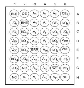
Figure 5. 48-ball VFBGA pinout (Single Chip Enable with ERR), CY62147GE  $^{[6,\ 7]}$
