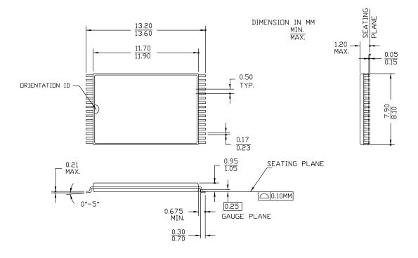
Figure 13. 32-pin Small TSOP (8 × 13.4 × 1.2 mm) ZA32, 51-85094
