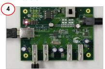
Connect a USB device to any of the four downstream ports. Use jumpers J7 to J10 in position 2-3 to enable the corresponding ports status LEDs. The red LED glowing indicates that the hub is not in Suspend mode. The green LED glowing indicates that the respective downstream port is enabled.
