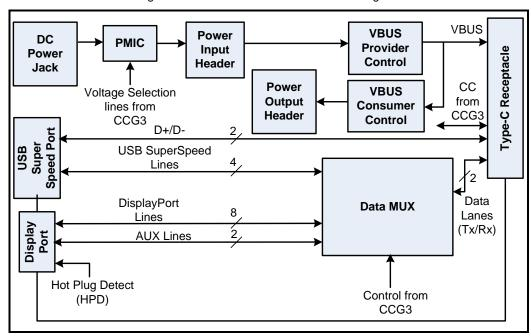
Figure 3-2: CCG EVK Base Board Block Diagram
