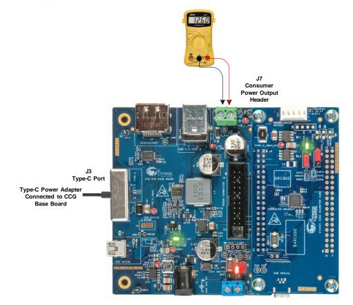
5. When the CCG3 device in the EVK is powered, it establishes a power contract with the Type-C power adapter and starts consuming power. This can be verified by connecting a digital multimeter to the consumer power output header (J7) of the CCG base board to measure the output voltage in the dead battery charging scenario. The output voltage at
