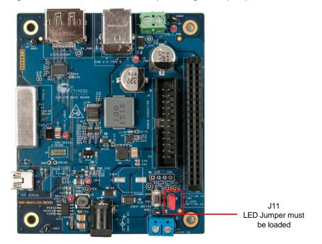
Figure 5-1: CCG EVK Base Board Jumper Settings for SuperSpeed USB Demo
