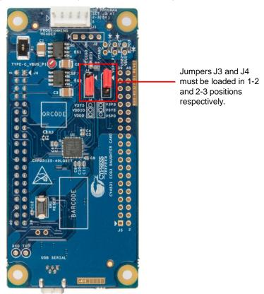
2. Mount the CCG3 daughter card on the CCG base board of the CY4531 EZ-PD CCG3 EVK if not already mounted. Use the SuperSpeed USB Type-A to Type-B cable to connect the CCG base board to the PC.
