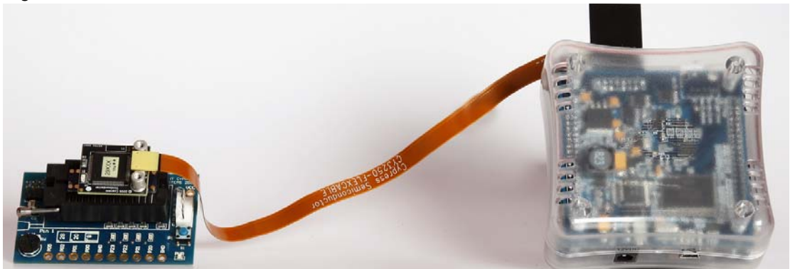
Figure 3-10. Flex Pod Connected to ICE-Cube Pod
