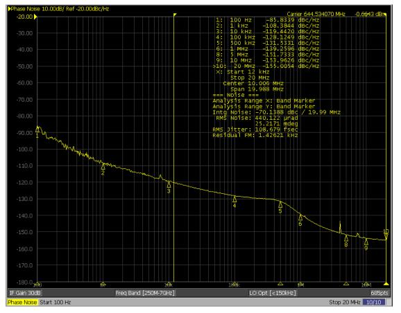
Figure 16. Typical Phase Noise at 644.53 MHz (12 kHz-20 MHz)
