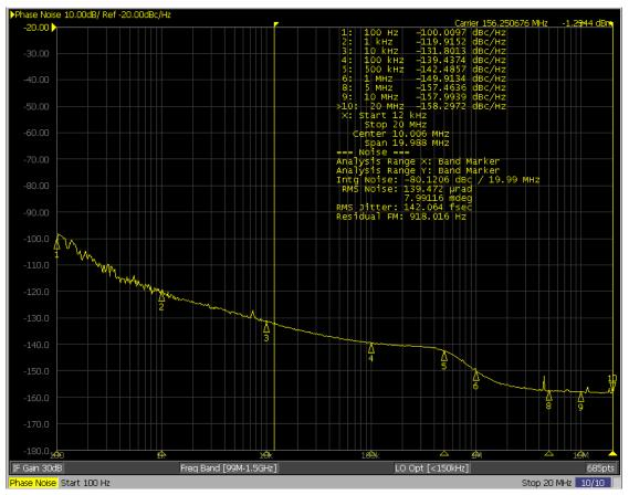
Figure 14. Typical Phase Noise at 156.25 MHz (12 kHz–20 MHz)
