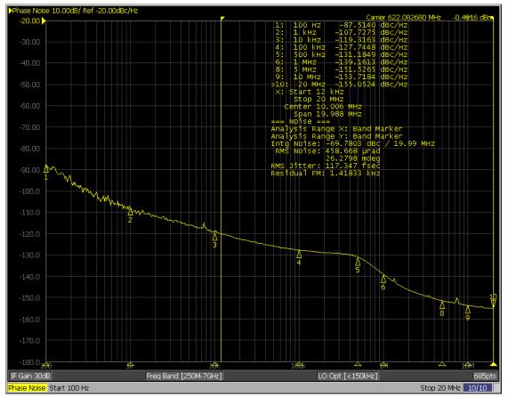
Figure 15. Typical Phase Noise at 622.08 MHz (12 kHz–20 MHz)
