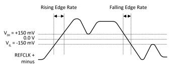
Figure 12. HCSL: Differential Measurement Points for Ringback
