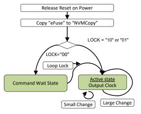
When the LOCK is programmed to "10" or "01", the device will go to the "Active state" and the device will perform at the programmed frequency.
