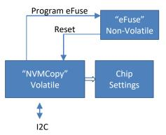
Figure 2 shows the conceptual internal memory structure that consists of Frequency Profile and Common Device Configuration settings.
