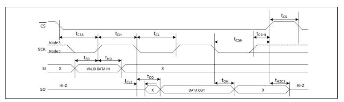
Figure 22 Synchronous data timing (Mode 0 and Mode 3)
