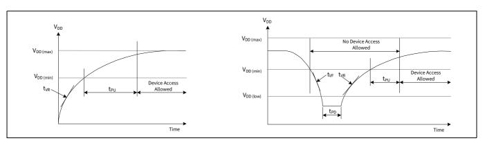
Figure 24 Power cycle timing
