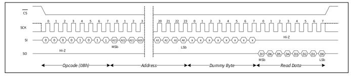
Figure 12 Fast read operation
