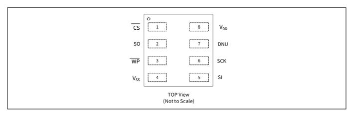
Figure 1 8-pin GQFN/UFLGA pinout
