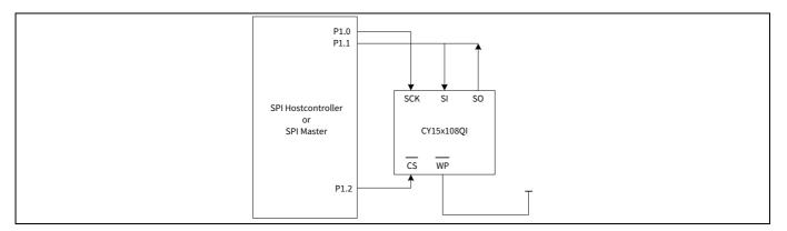
Figure 3 System configuration without SPI port
