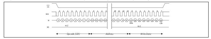
Figure 10 Memory write (WREN not shown) operation
