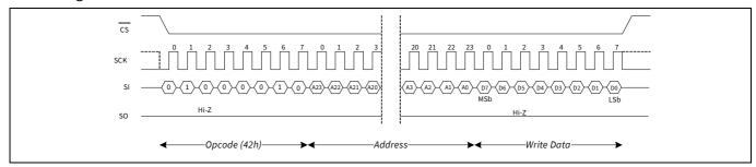
Figure 13 Special sector write (WREN not shown) operation
