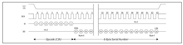
Figure 18 Read serial number operation
