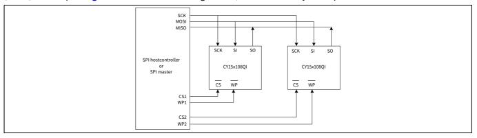
Figure 2 System configuration with SPI port
