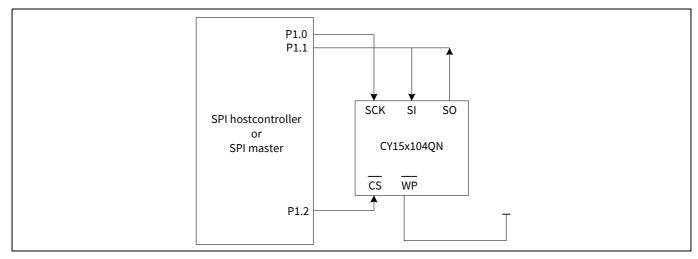
Figure 4 System configuration without SPI port
