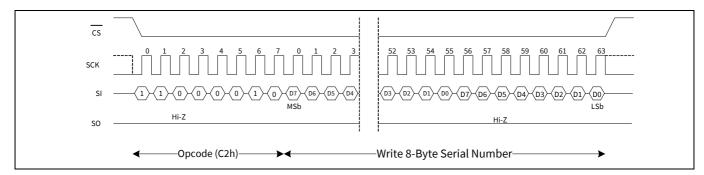
Figure 18 Write serial number (WREN not shown) operation
