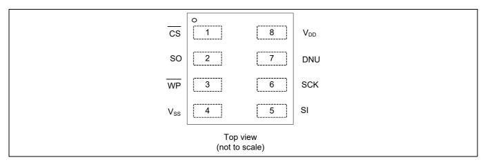
Figure 1 8-pin GQFN/UFLGA pinout
