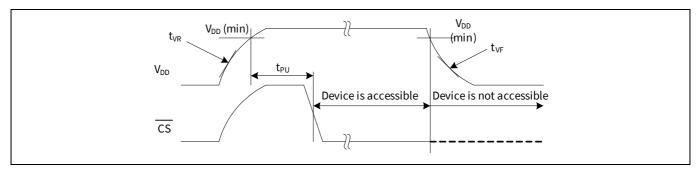
Figure 25 Power cycle timing
