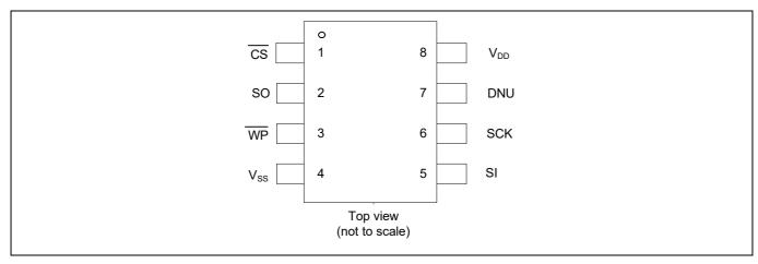
Figure 2 8-pin SOIC pinout
