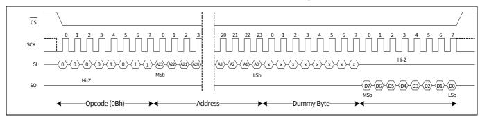
Figure 13 Fast read operation
