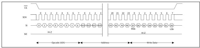
Figure 14 Special sector write (WREN not shown) operation
