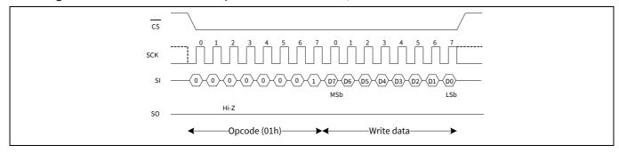
Figure 10 WRSR bus configuration (WREN not shown)
