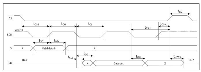
Figure 23 Synchronous data timing (Mode 0 and Mode 3)
