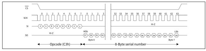
Figure 19 Read serial number operation
