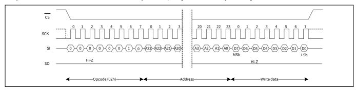
Figure 11 Memory write (WREN not shown) operation
