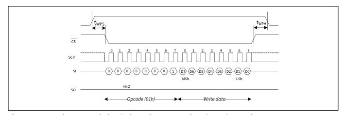
Figure 24 Write protect timing during write status register (WRSR) operation
