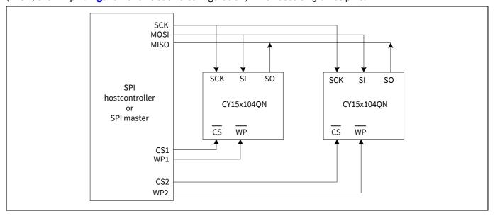
Figure 3 System configuration with SPI port
