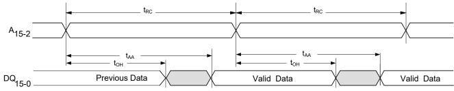
Figure 6. Read Cycle Timing No. 2 (CE Controlled)
