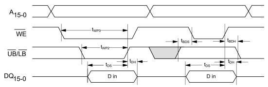
Figure 12. Page Mode Write Cycle Timing
