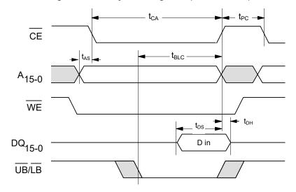
Figure 10. Write Cycle Timing No. 3 ( $\overline{\text{CE}}$  LOW) [8]
