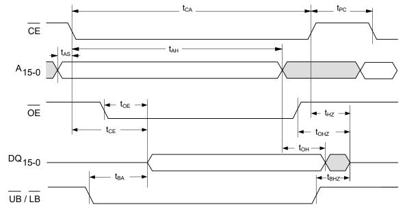
Figure 7. Page Mode Read Cycle Timing  $^{[7]}$
