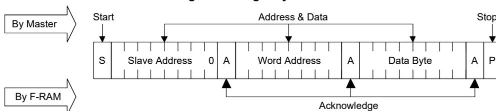
Figure 8. Multi-Byte Write
