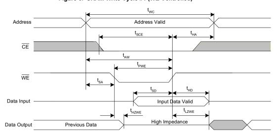
Figure 7. SRAM Write Cycle #2 ( $\overline{\text{CE}}$  Controlled) [19, 20, 21]
