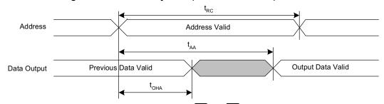
Figure 5. SRAM Read Cycle #2 ( $\overline{\text{CE}}$  and  $\overline{\text{OE}}$  Controlled) [16, 18]
