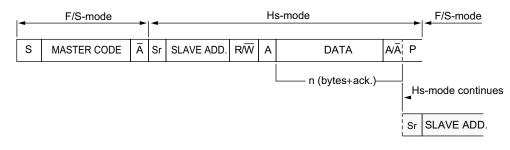
Single and multiple-byte reads and writes are supported. After the device enters into Hs-mode, data transfer continues in Hs-mode until stop condition is sent by master device. The slave switches back to F/S-mode after a STOP condition (P). To continue data transfer in Hs-mode, the master sends Repeated START (Sr).
