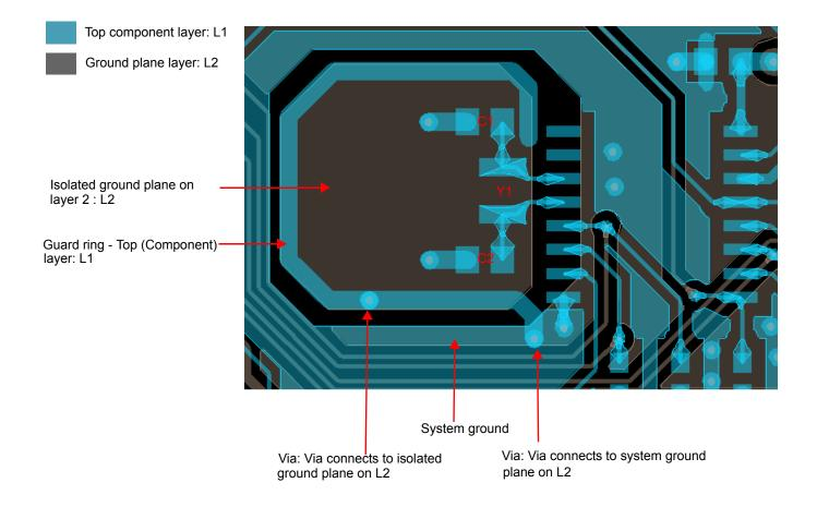
Figure 39. Recommended Layout for RTC
