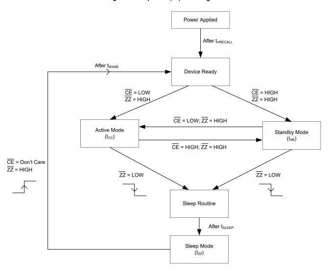
Figure 5. Sleep Mode (ZZ) Flow Diagram
