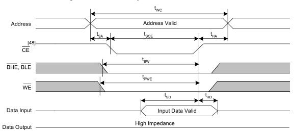
Figure 15. SRAM Write Cycle 2: CE Controlled[44, 45, 46, 47]
