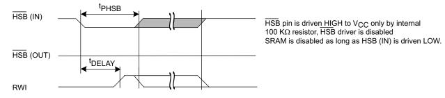
Figure 22. Soft Sequence Processing<sup>[64, 65]</sup>
