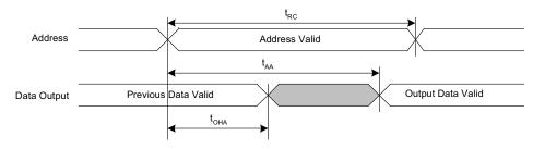
Figure 12. SRAM Read Cycle 2:  $\overline{\text{CE}}$  and  $\overline{\text{OE}}$  Controlled<sup>[34, 36, 37]</sup>
