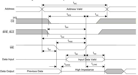
Figure 13. SRAM Write Cycle 1:  $\overline{\text{WE}}$  Controlled<sup>[39, 40, 41, 42]</sup>
