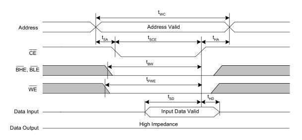
Figure 9. SRAM Write Cycle #2 (CE Controlled) <sup>[36, 37, 38, 39]</sup>
