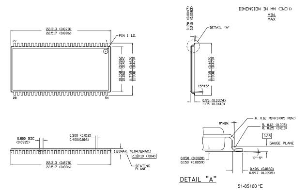
Figure 20. 54-pin TSOP II (22.4 × 11.84 × 1.0 mm) Package Outline, 51-85160
