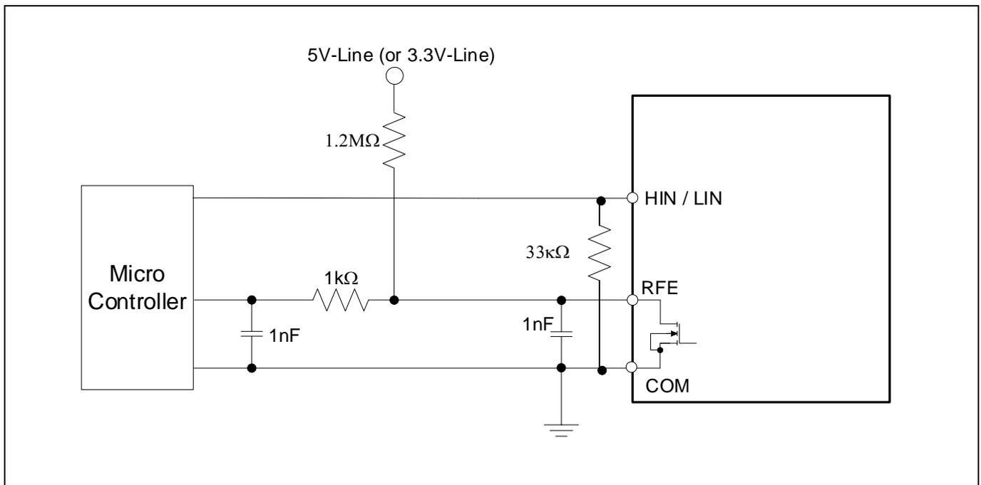
**Figure 17** Recommended microcontroller I/O interface circuit
