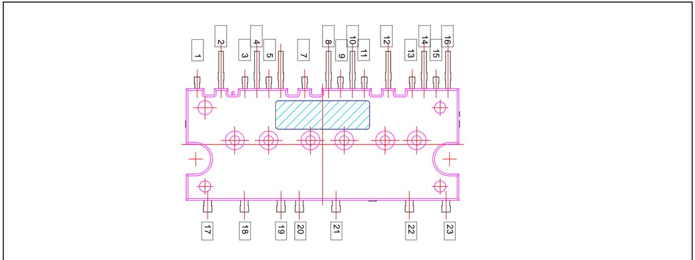
Figure 4 Module pinout
