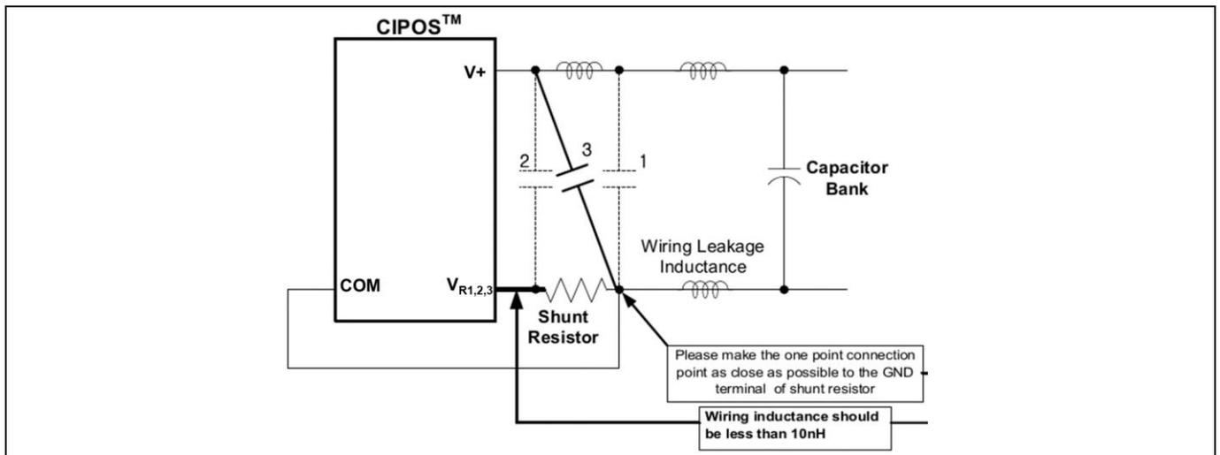
**Figure 20** Proper snubber capacitor use
