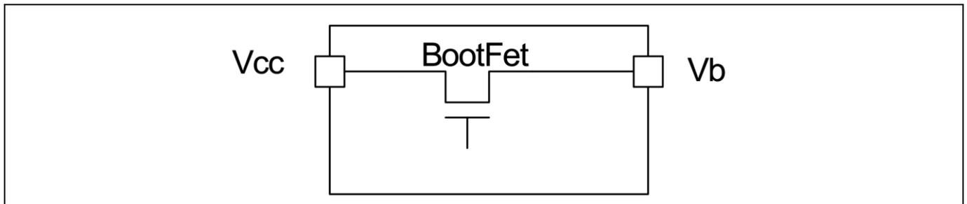
Figure 22 Simplified BootFET internal connection
