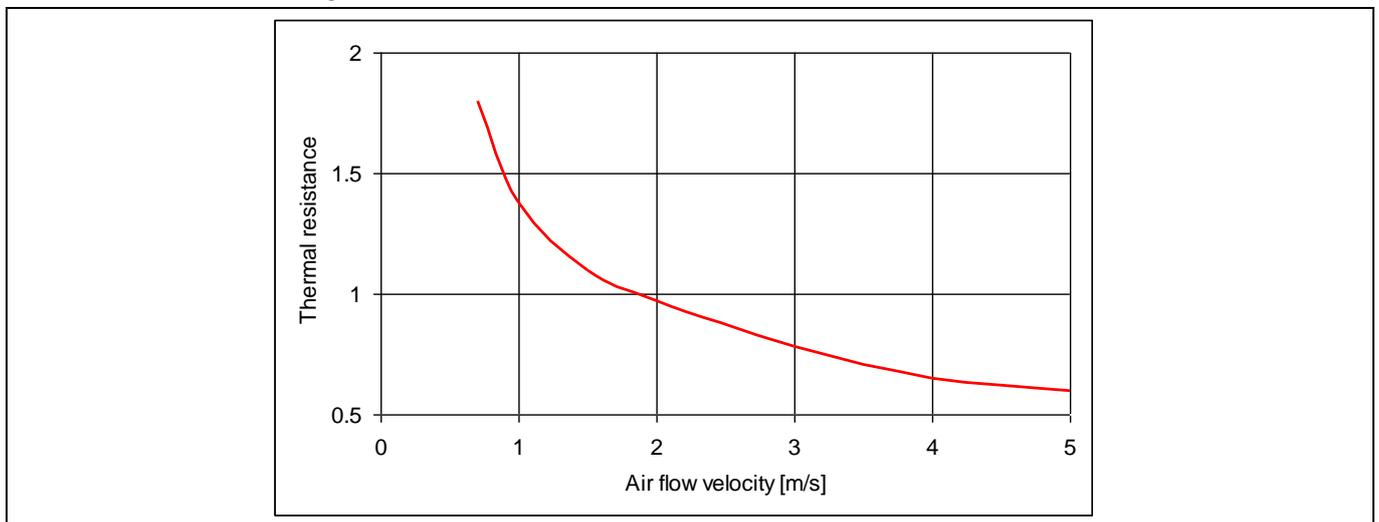
**Figure 30** Thermal resistance vs. air flow velocity
