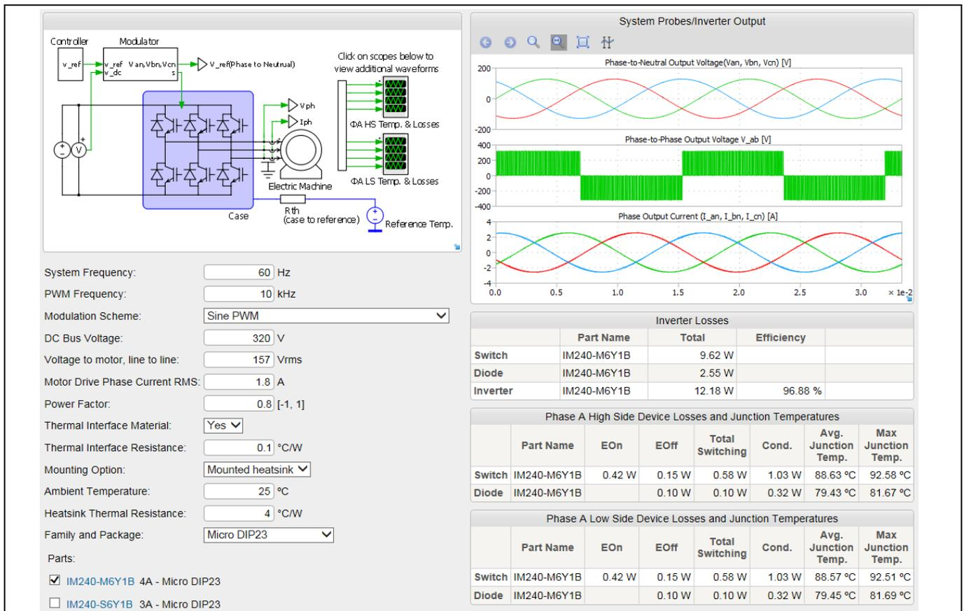
**Figure 26** CIPOS™ IPM motor-drive-simulation tool example for IM240-M6Y1B
