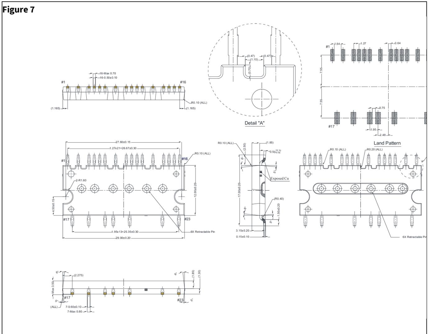
Figure 8 SOP 29x12 (dimensions in mm)
