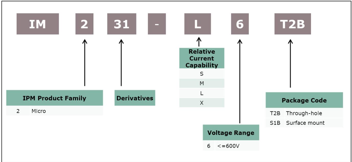
**Figure 1** Nomenclature for CIPOS™ Micro IPM's IM231 series
