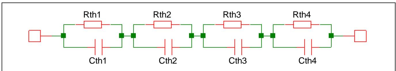
**Figure 27** Thermal impedance RC equivalent circuit (Foster model)
