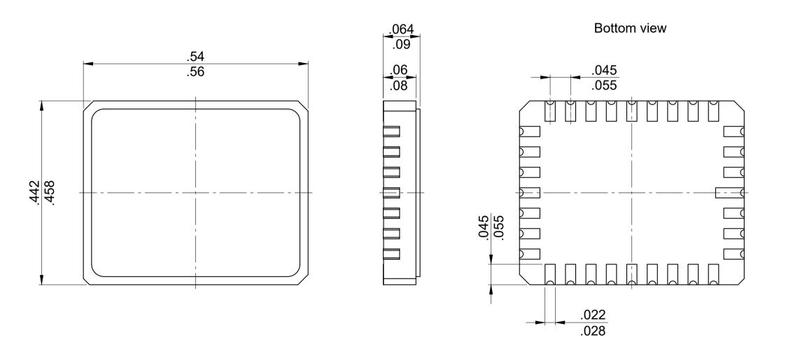
All dimensions are in units inches  $\frac{\text{min.}}{\text{max.}}$ The drawing is in compliance with ISO 128-30, Projection Method 1 [
