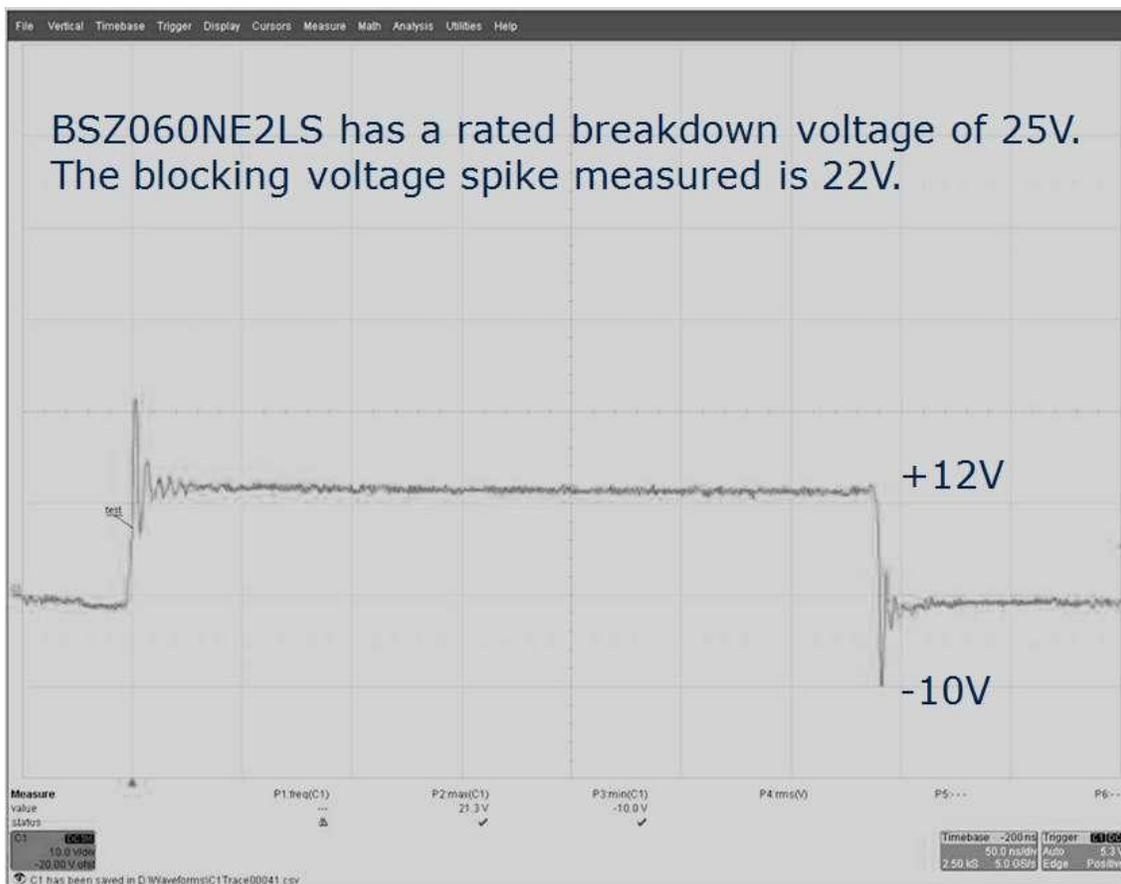
Figure 5 Measured spike
