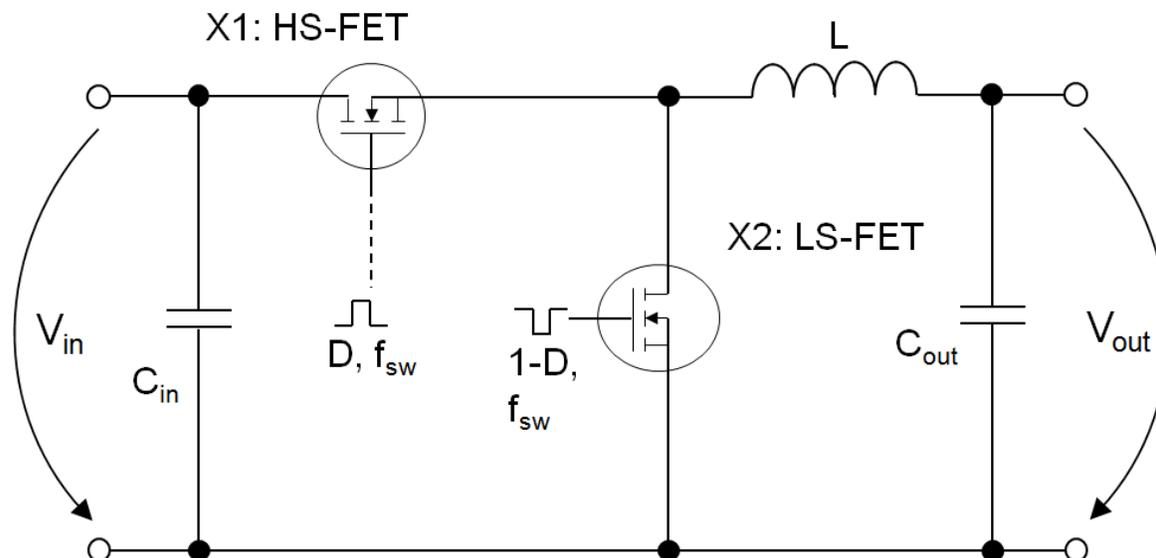
**Figure 1 Standard buck-converter with synchronous rectification**
