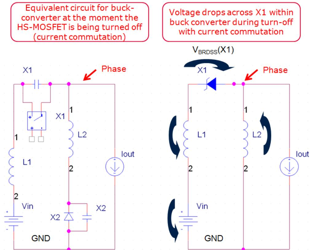
**Figure 3 Analysis schematic for negative spike event**
