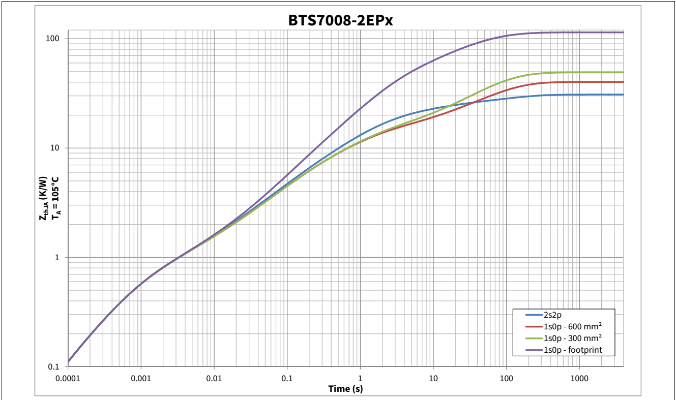
Figure 9 Typical Thermal Impedance. PCB setup according Chapter 4.4.1
