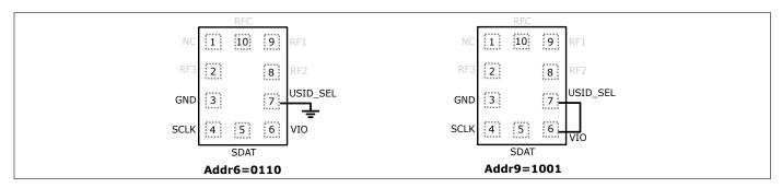
Figure 4: BGSC2341ML10 USID\_SEL Pin Configuration
