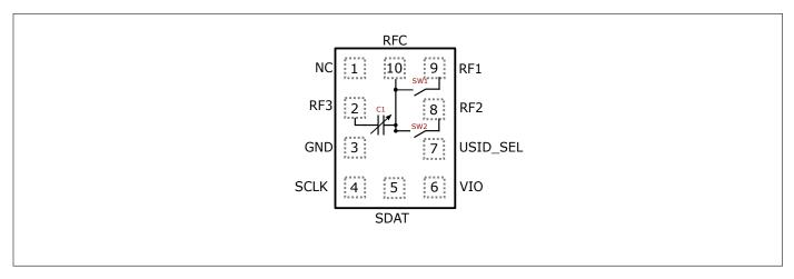
Figure 5: BGSC2341ML10 Pin Configuration (top view)
