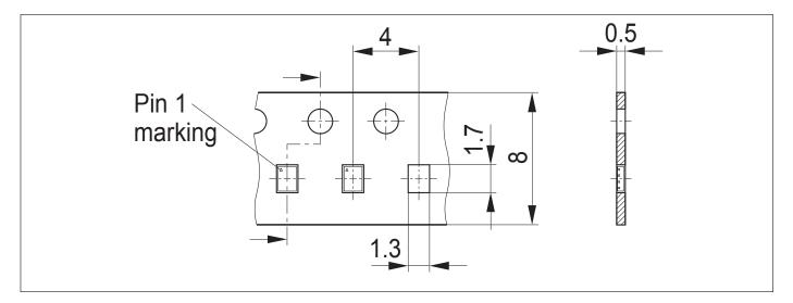
Figure 9: TSLP-10-2 Carrier Tape
