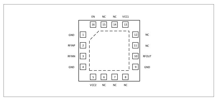
Figure 2: BGAP2D20A Pin Configuration - Top View
