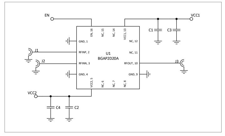
Figure 3: BGAP2D20A Application Schematic
