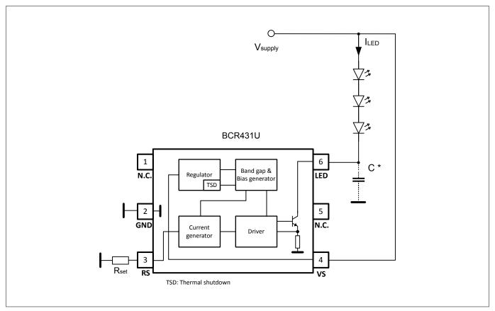
Figure 1 Typical Application Circuit of BCR431U
