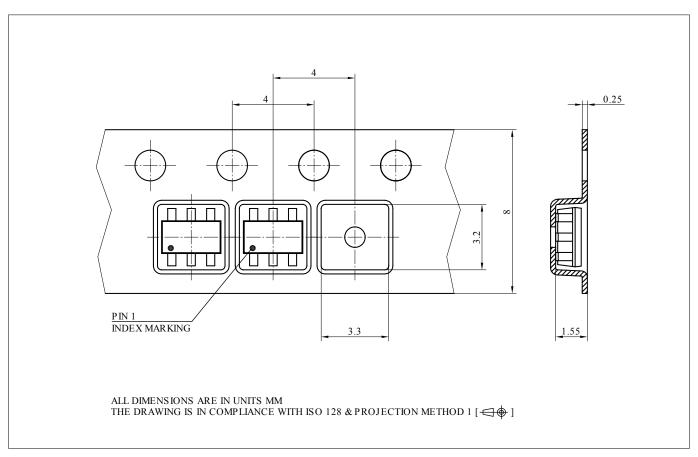
Figure 8 Tape & Reel PG-SOT23-6
