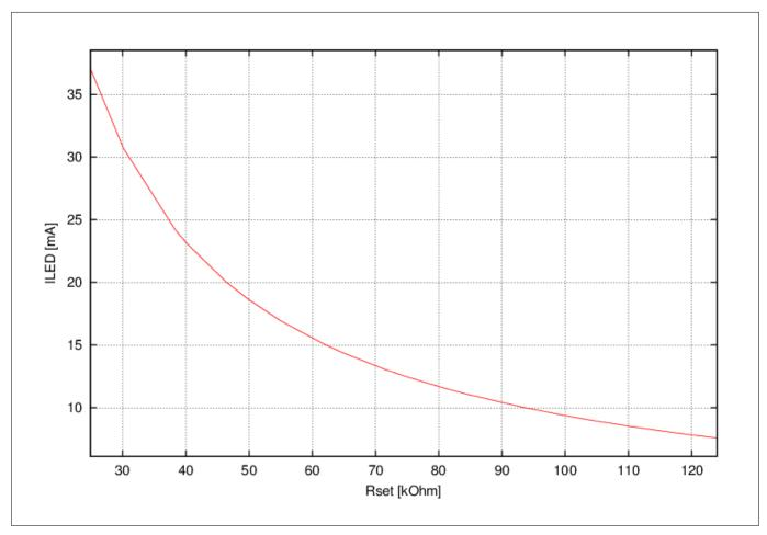
Figure 3 Relation between  $I_{LED}$  and  $R_{set}$
