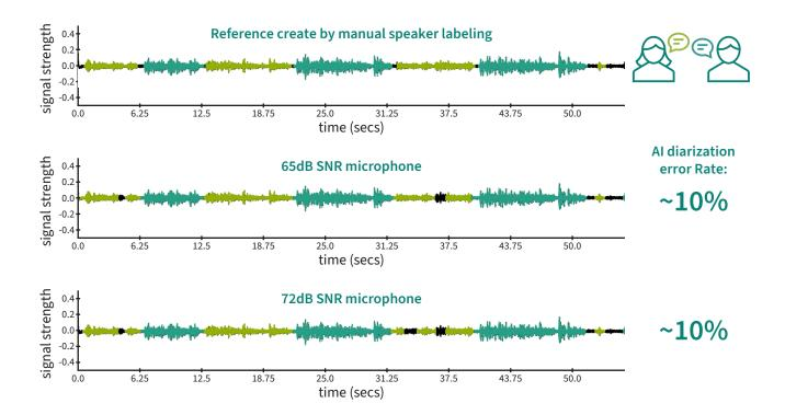
The two graphs show the reference with the audio sequence of the first speaker in green and the audio sequence of the second speaker in turquese. The reference was given to NeMo by manual labeling. Each time a specific button was pressed at each turn of the speaker.
