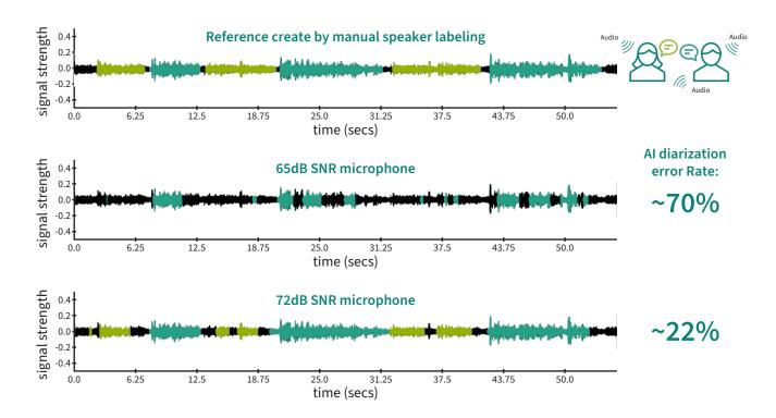
With background noise, NeMo struggled to even detect the second speaker when the recording was done with the medium SNR microphone. The diarization error rate showed up as around 70%.
