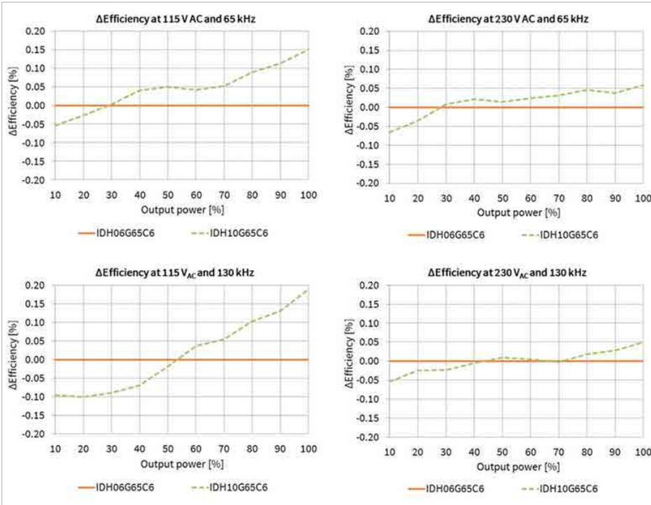
Figure 2: Measured efficiency of the 800 W PFC board - different current rating full load conditions. The design improvements have introduced a lower forward voltage ( $V_f$ ) in the new CoolSiC™ Schottky diode 650 V G6 diode which results in temperatures (measured and simulated) that are around 1 °C lower after 100  $\mu$ s than the previous generation diode (CoolSiC™ Schottky diode 650 V G5).
