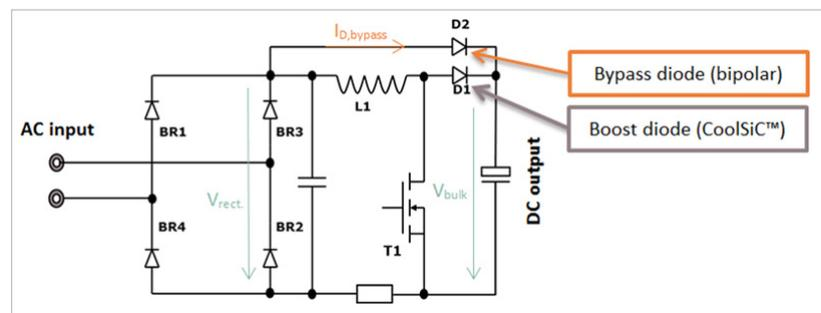
Figure 3: Simplified classic PFC circuit diagram with a bypass diode
