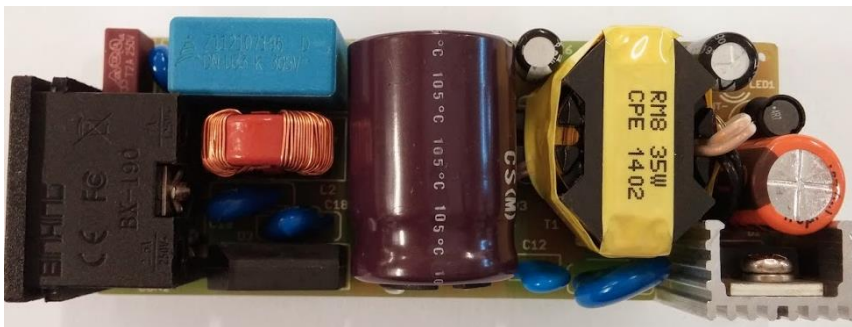
Figure 2A – REF-ICE2QS03G & IPD60R600P6 35W ADAPTER (Top Side)
