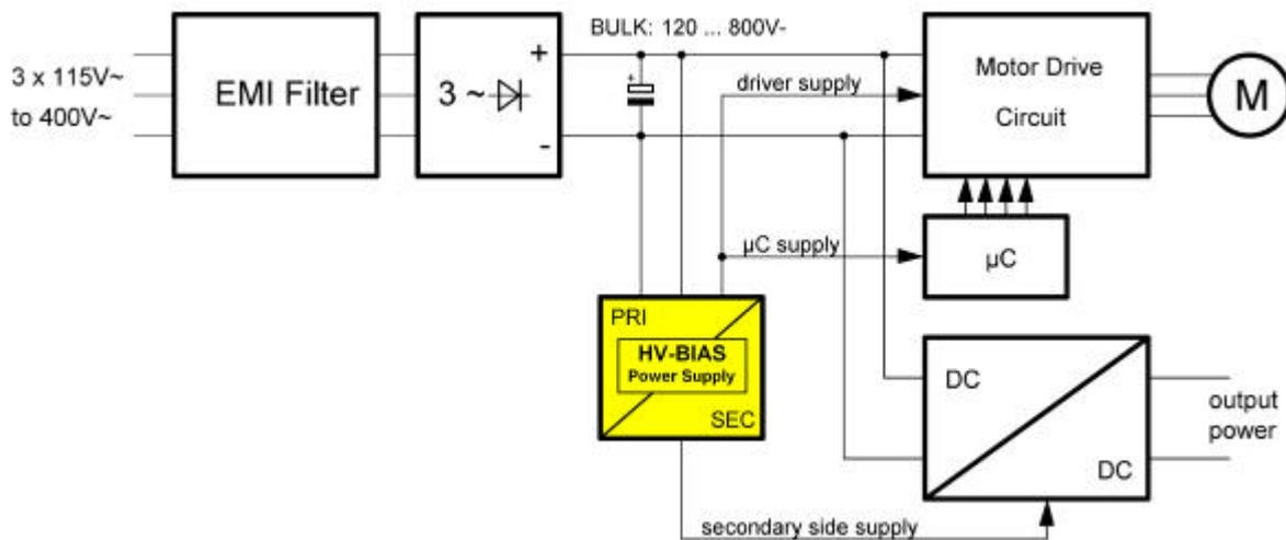
Figure 1: Principle application of the HV-Bias circuit
