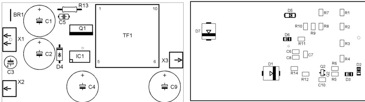
Figure 10: Components placement on the top (left) and the bottom (right) side
