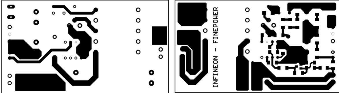
Figure 9: Layout TOP - left and BOTTOM (mirrored) – right
