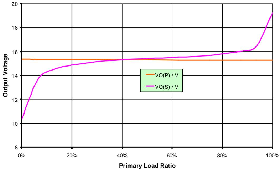
Fig. 5: Cross Regulation while secondary side is shunted with 1k?
