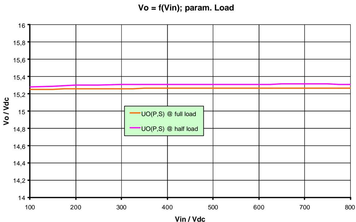
Figure 4: Line Regulation at half and full load
