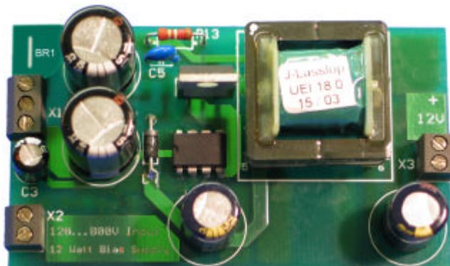
Figure 8: The HV-Bias Module – nearly original size
