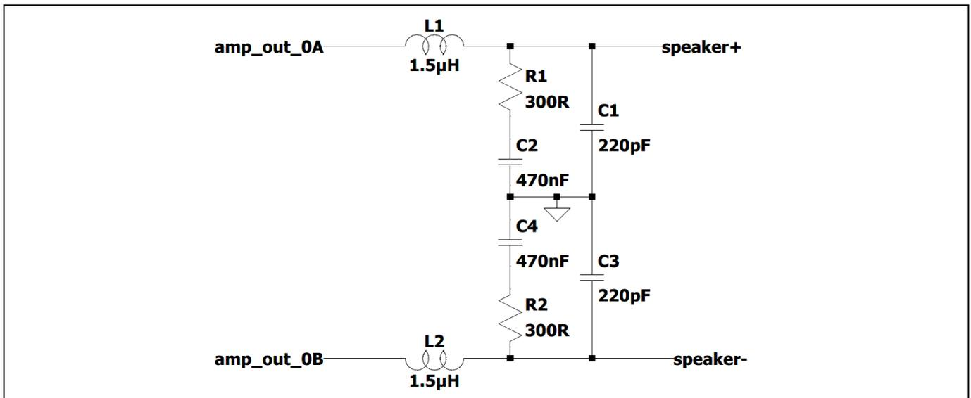
**Figure 5 LC output filter configuration 2 with damping filter for 1x1BT output**
