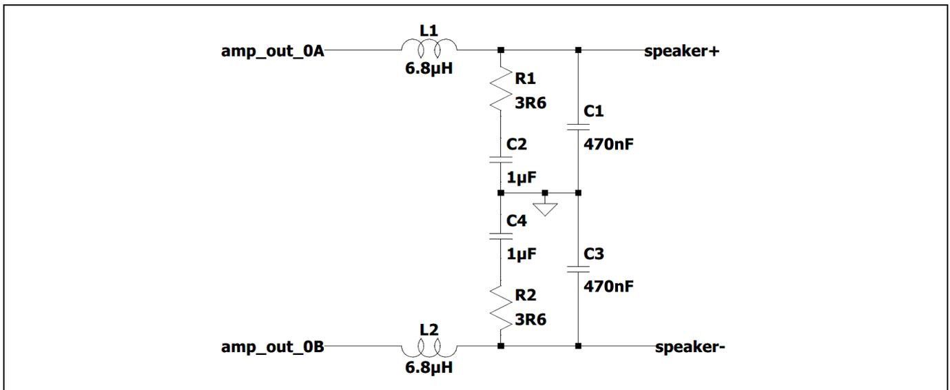
**Figure 6** LC output filter configuration 3 with damping filter for 1x BTL output
