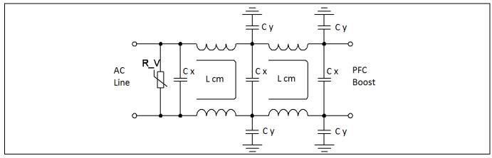
Figure 4 Two stage filter structure
