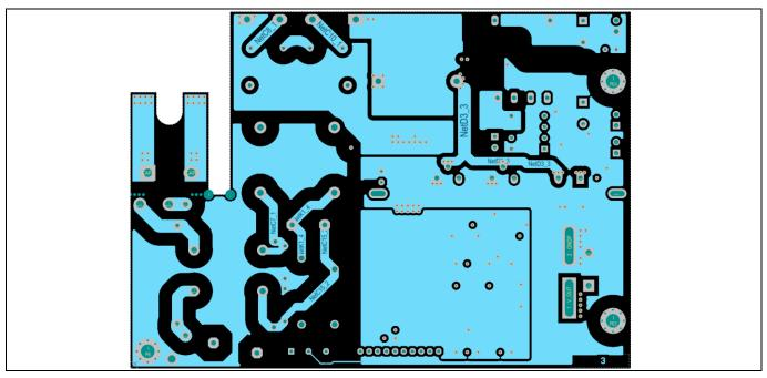
Figure 31 View of PCB inner 2 layer
