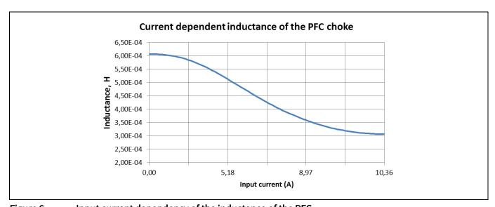
Figure 6 Input current dependency of the inductance of the PFC
