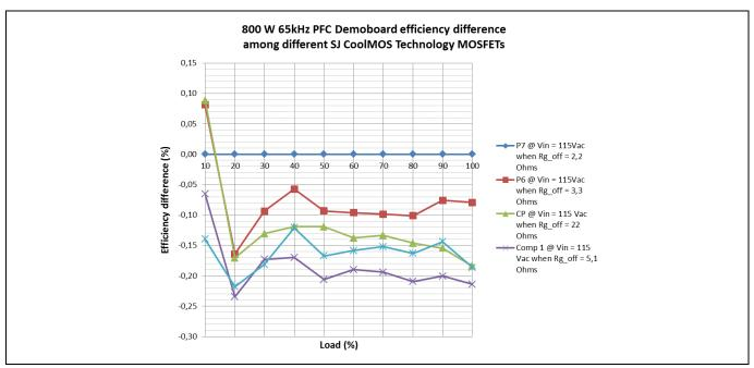
Figure 17 Efficiency difference among selected SJ MOSFETs from Infineon and closest competitors with  $R_{DS\ ON}$  close to 180 m $\Omega$ .
