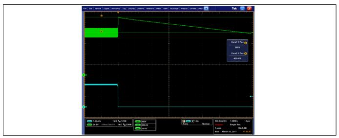
Figure 20 Load step:  $100\% \rightarrow 0\%$  at  $V_{IN} = 115 \text{ V AC}$
