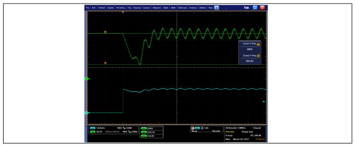
Figure 18 Load step:  $0\% \rightarrow 100\%$  at  $V_{IN} = 115 \text{ V AC}$
