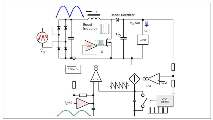
Figure 7 Simplified block diagram concept for PFC PWM modulator of the ICE3PCS0x series
