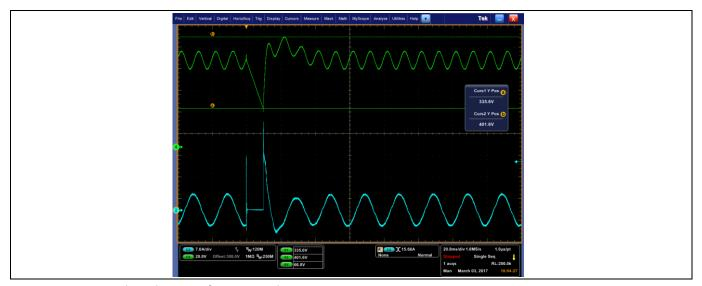
Figure 24 AC line drop out for 10 ms when  $V_{IN} = 230 \text{ V AC}$  at  $P_{OUT} = 800 \text{ W}$
