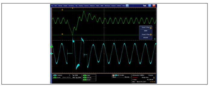
Figure 23 AC line drop out for 10 ms when  $V_{IN} = 115 \text{ V AC}$  at  $P_{OUT} = 800 \text{ W}$
