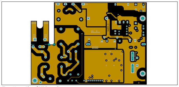
Figure 30 View of PCB inner 1 layer
