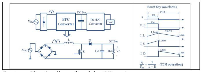
Figure 1 Schematics and key waveforms of a boost PFC converter
