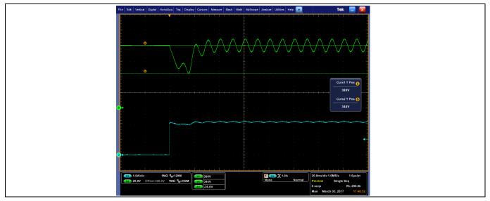
Figure 19 Load step:  $0\% \rightarrow 100\%$  at  $V_{IN} = 230 \text{ V AC}$
