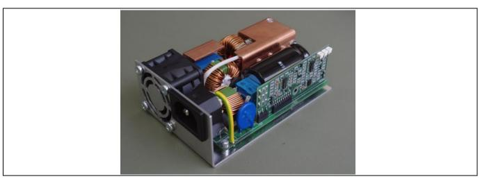
Figure 25 Picture of the 800 W 65kHz PFC demo board
