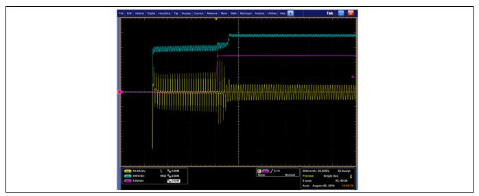
Figure 22 Start-up at  $V_{IN} = 230 \text{ V DC}$
