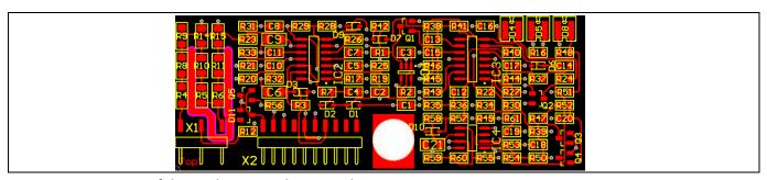
Figure 36 View of the analog control PCB top layer
