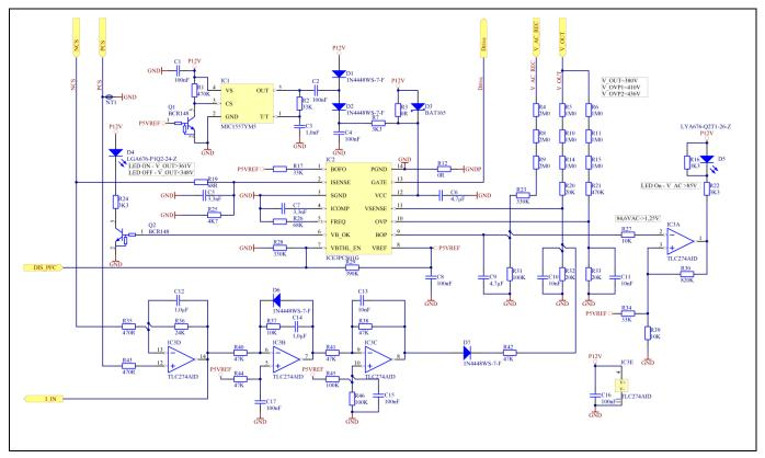
Figure 34 Schematic of PFC control
