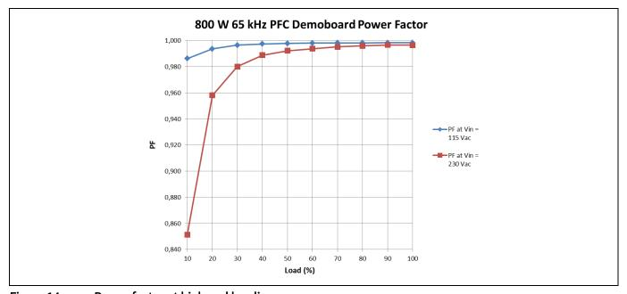
Figure 14 Power factor at high and low line
