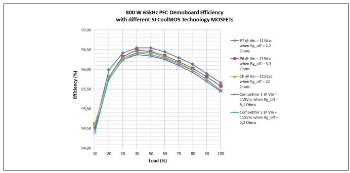
Figure 16 Efficiency comparison at  $V_{IN}$  = 115 V AC among selected SJ MOSFETs from Infineon and closest competitors with  $R_{DS\_ON}$  close to 180 m $\Omega$ .
