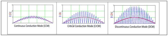
Figure 2 PFC inductor current and average input current in the three different operating modes
