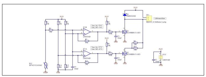
Figure 27 Schematic of fan control
