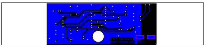
Figure 39 View of analog control PCB bottom layer
