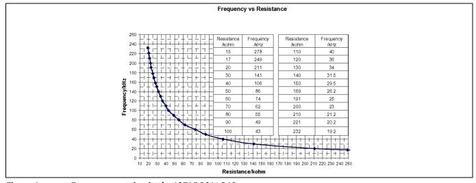
Figure 9 Frequency setting in the ICE3PCS01G IC
