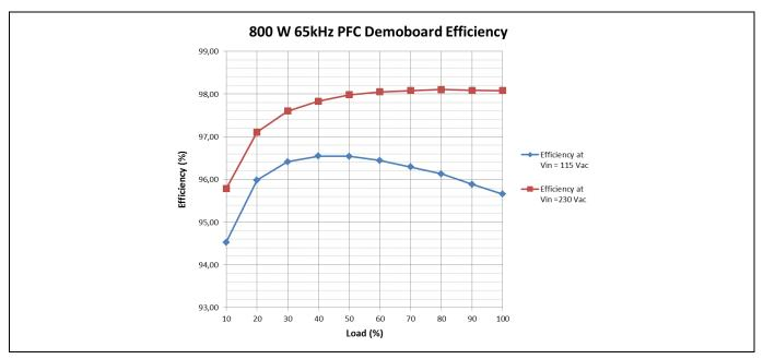
Figure 13 High and low line efficiency when  $R_{g_on} = 15 \Omega$  and  $R_{g_off} = 2.2 \Omega$
