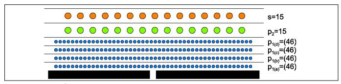
Figure 10 Winding arrangement
