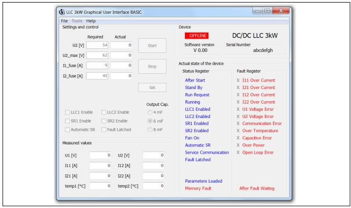
Figure 34 LLC 3 kW Graphical User Interface (GUI)
