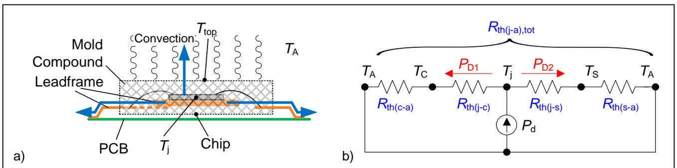
**Figure 1** a) Cross section through an IC and package
