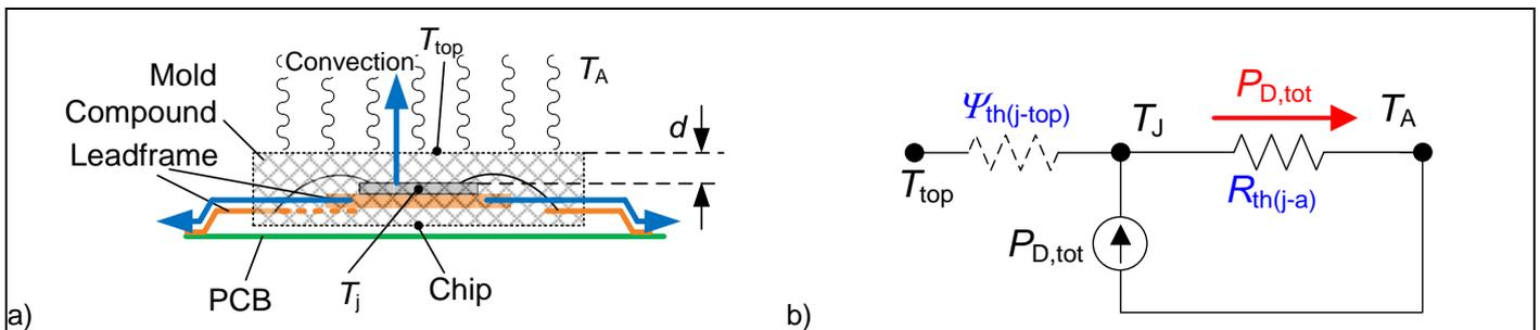
**Figure 2 a) Cross section through an IC and package for simplified heat flow path**
