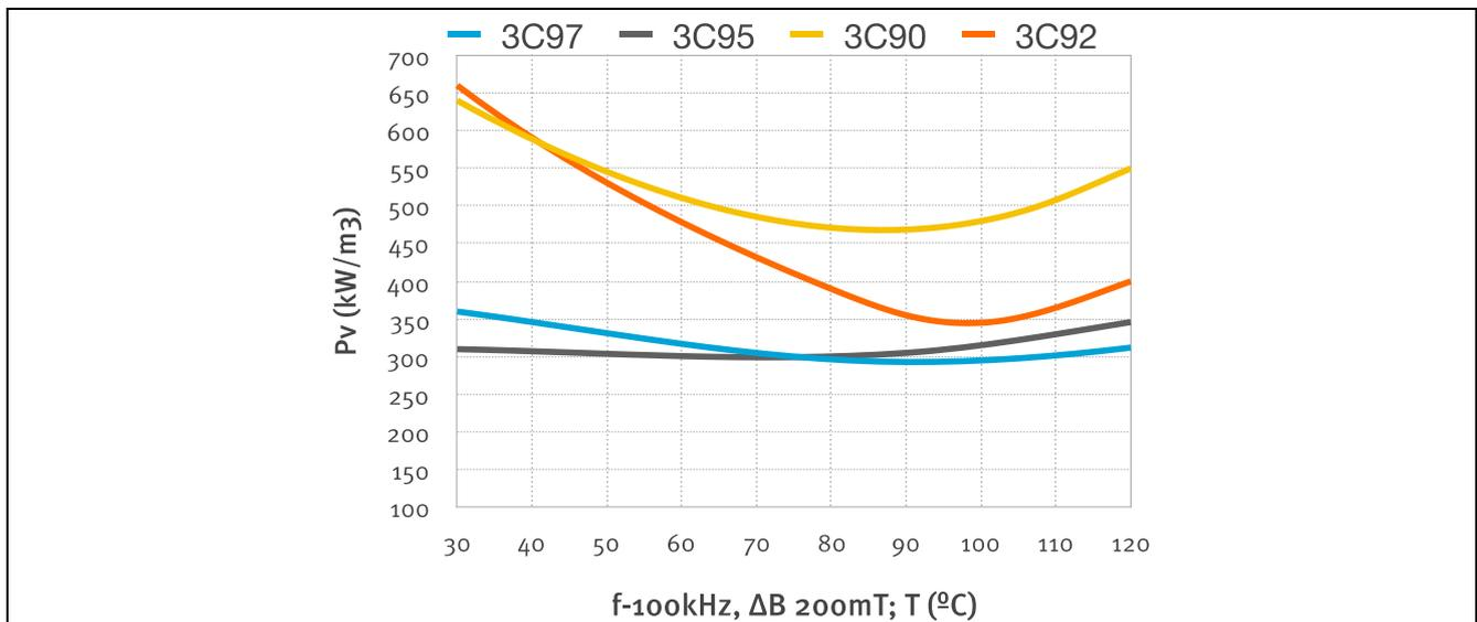
Figure 15 Ferrite core material TDK PC95/3C95
