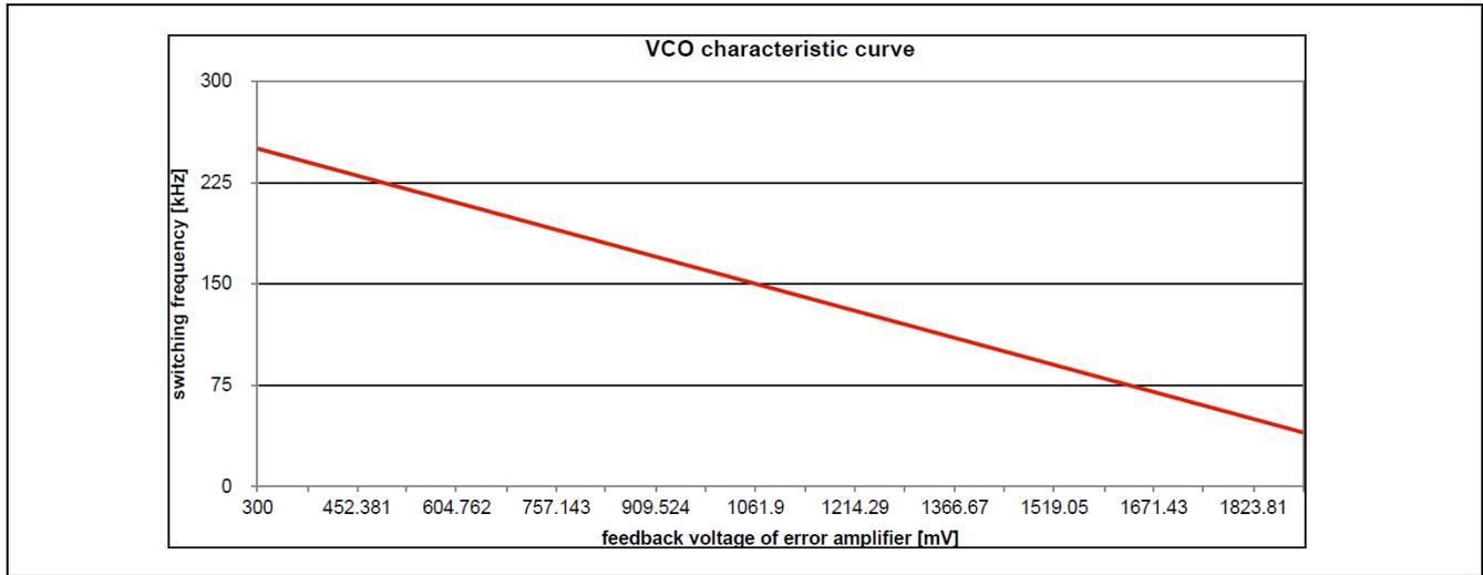
Figure 34 VCO characteristic curve:  $f_{SW}$  vs.  $V_{FREQ}$
