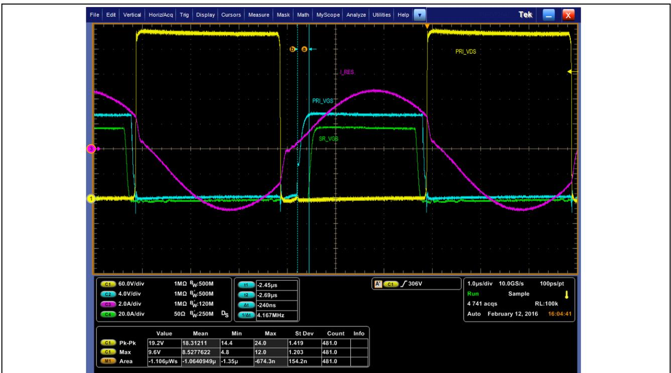
Figure 44 SR turn-on and turn-off delays above resonance
