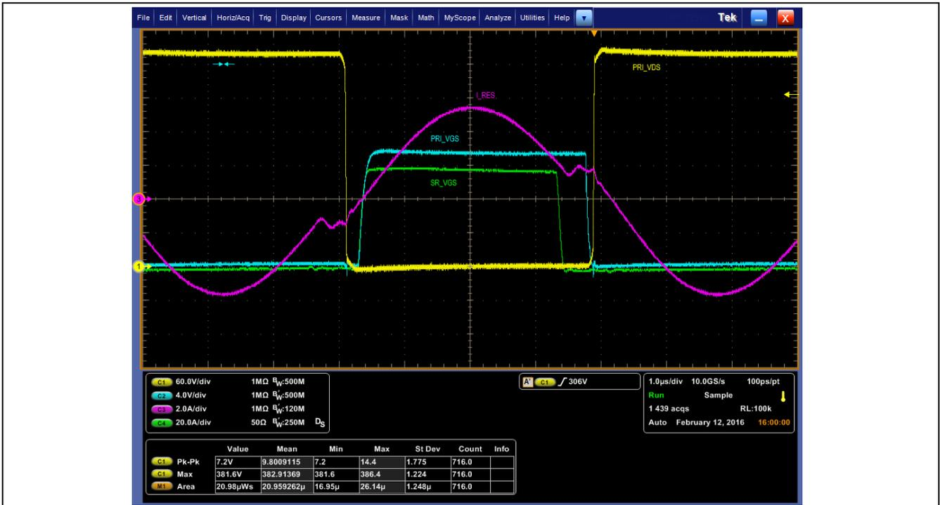
Figure 43 SR turn-on and turn-off delays below resonance
