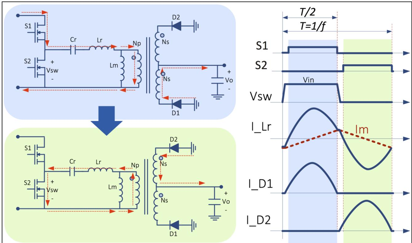
**Figure 4** Fully resonant operating mode, at the resonant point for C<sub>r</sub> and L<sub>r</sub>, with near ZCS turn-off of the primary side MOSFETs.
