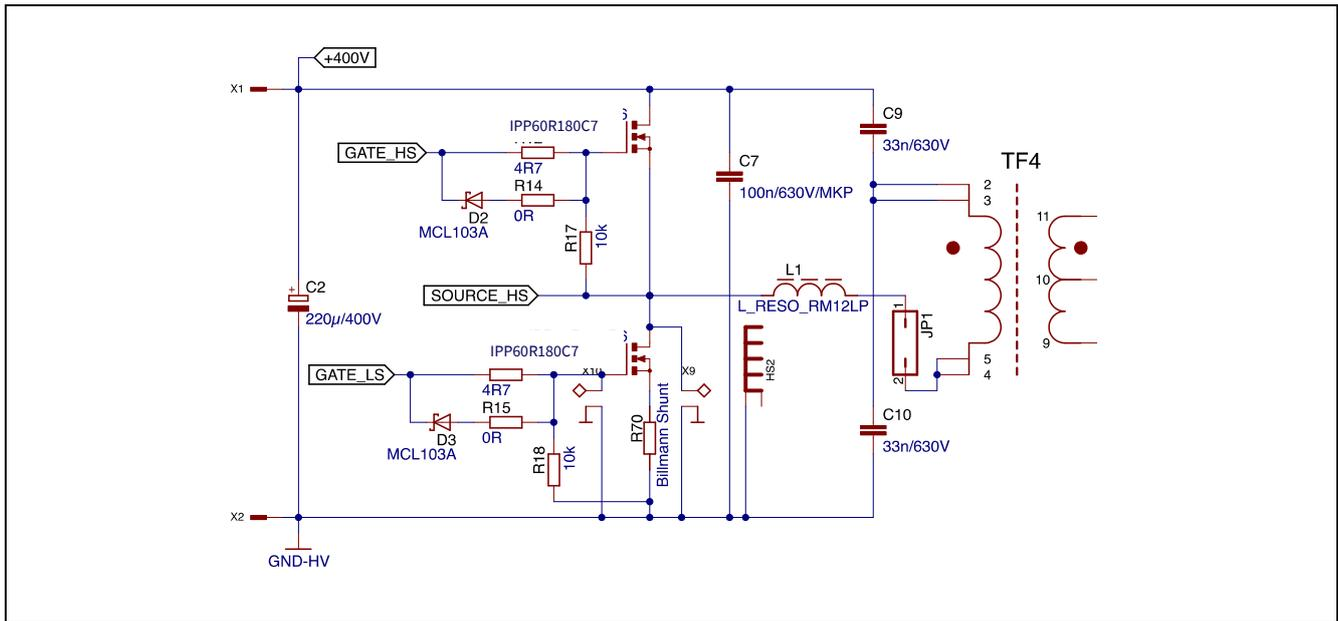
**Figure 22** HB C<sub>r</sub> capacitor configuration to reduce capacitive mode operation and distribute AC voltage stress between two capacitors
