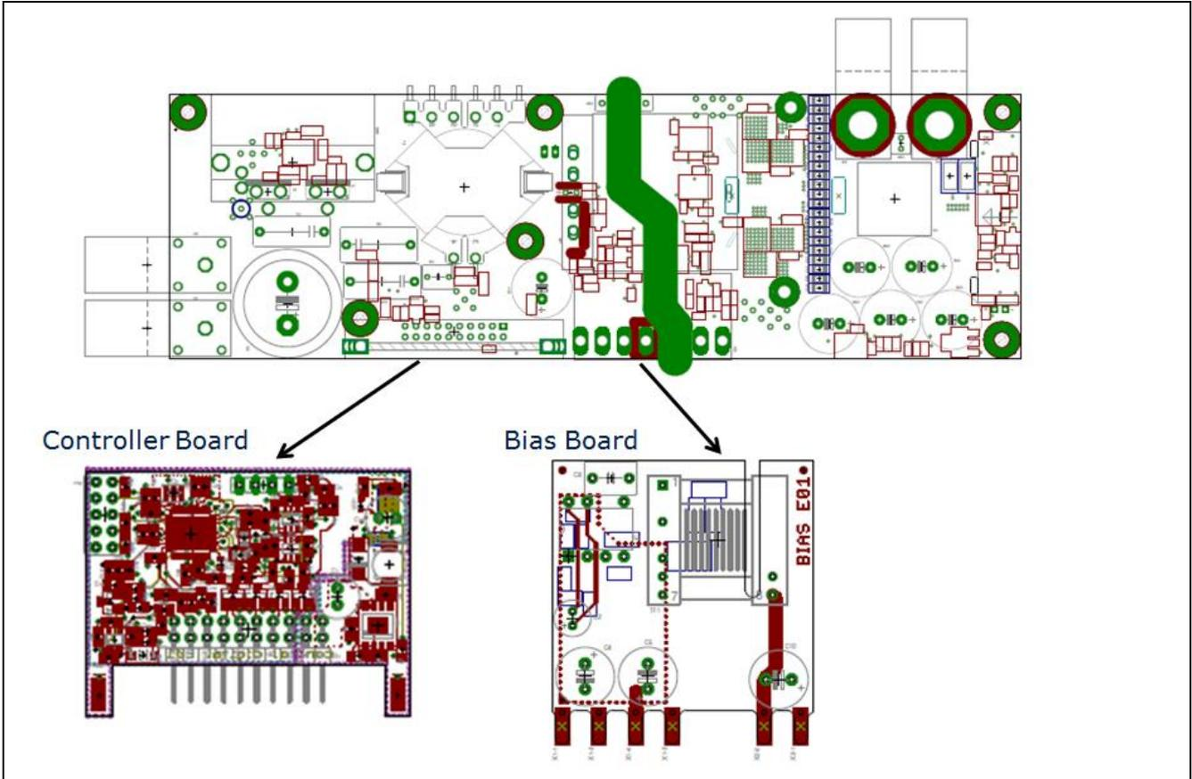
Figure 33 Mainboard PCB with controller – and biasboard
