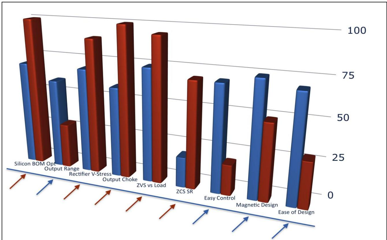
**Figure 1** Comparison of several Figure of Merit(FoM) metrics based on cost and performance between the ZVS PSFB converter (blue) and the LLC HB (red).
