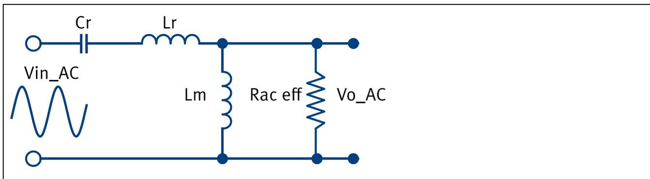
Figure 8 First harmonic approximation equivalent resonant circuit
