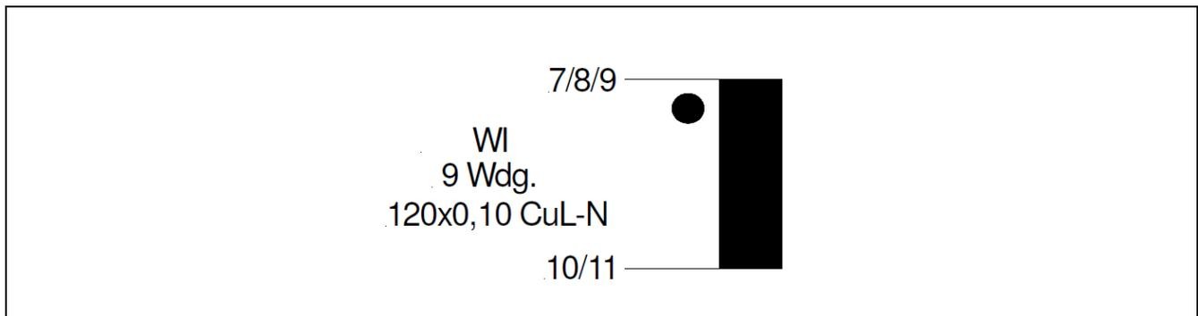
Figure 21 Winding structure of the RM 12 resonant choke (ICE Transformer s.r.l.)
