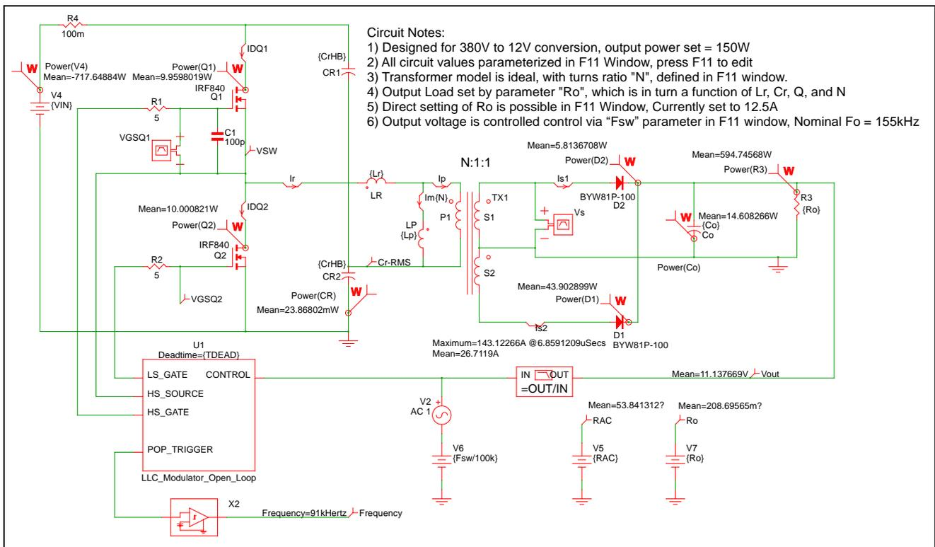
Figure 17 LLC open loop simulation circuit using SIMPLIS
