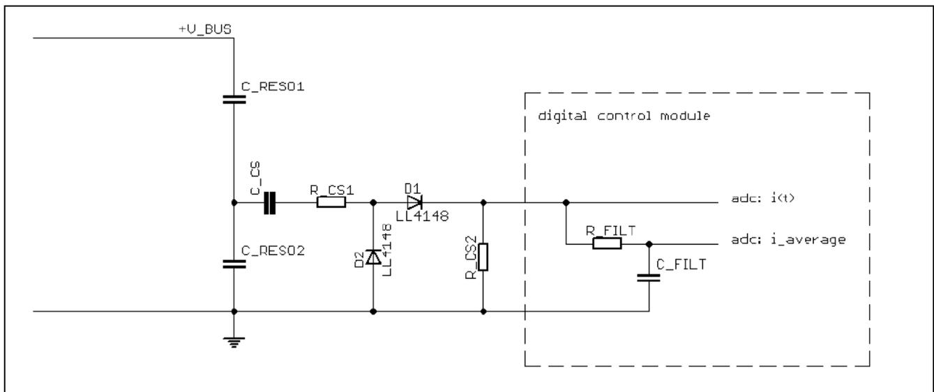
**Figure 46 Anti-capacitive load mode: instantaneous primary current measurement**
