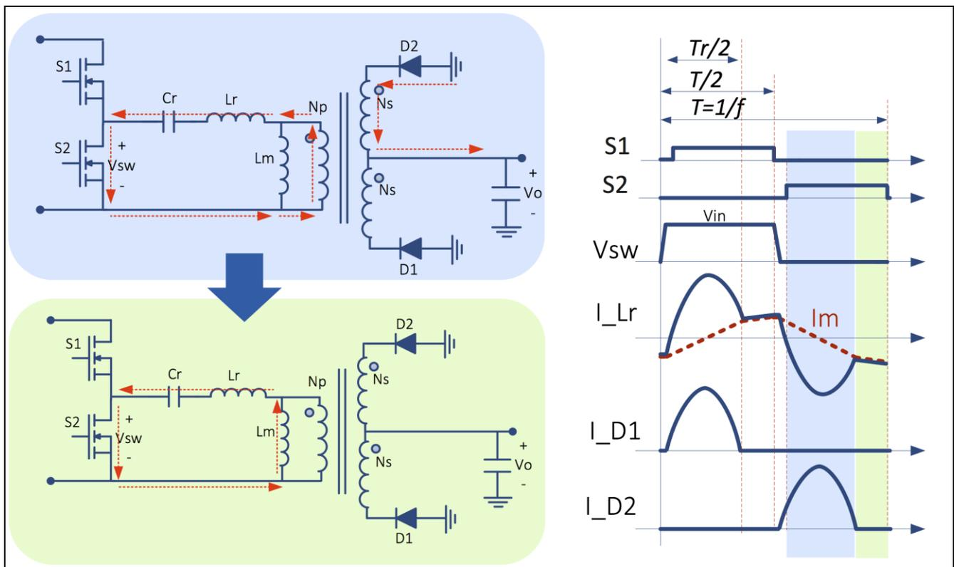
Figure 7 Under resonant DCM mode operation, (between resonant point of  $C_r$  and  $L_r$ , versus resonant point of  $C_r$  and  $L_r+L_m$ ) 2<sup>nd</sup> half cycle
