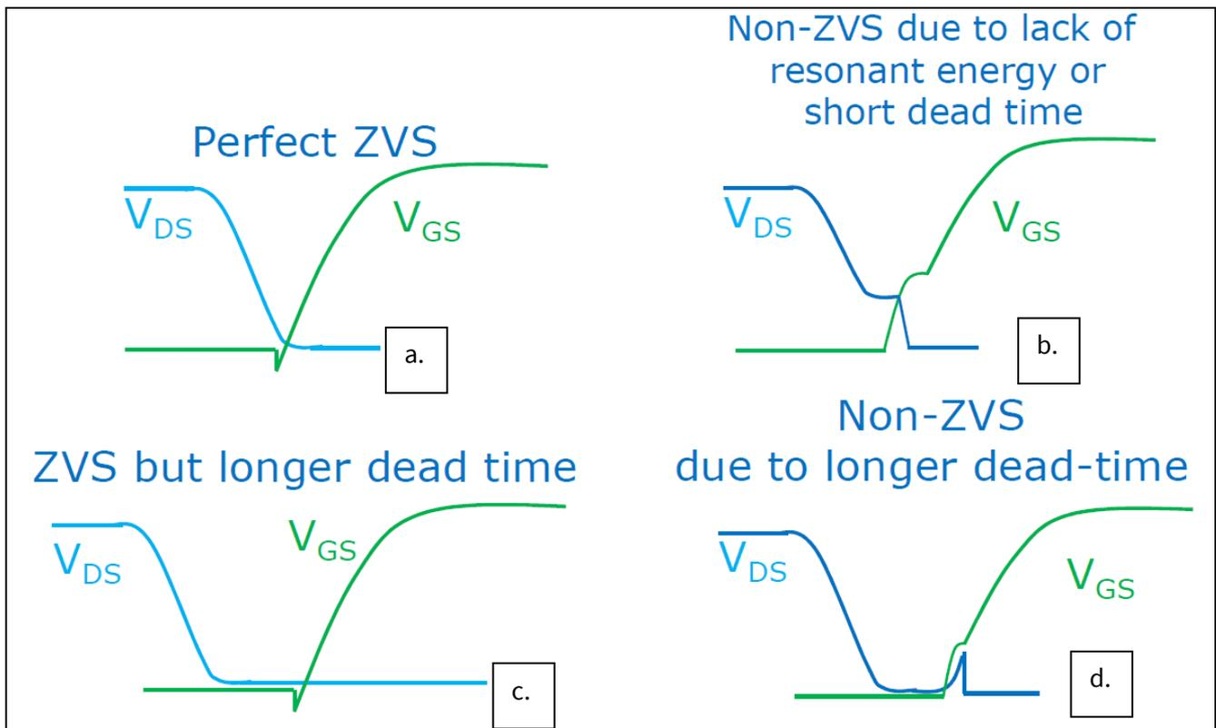
**Figure 40** Proper and wrong dead time setting.
