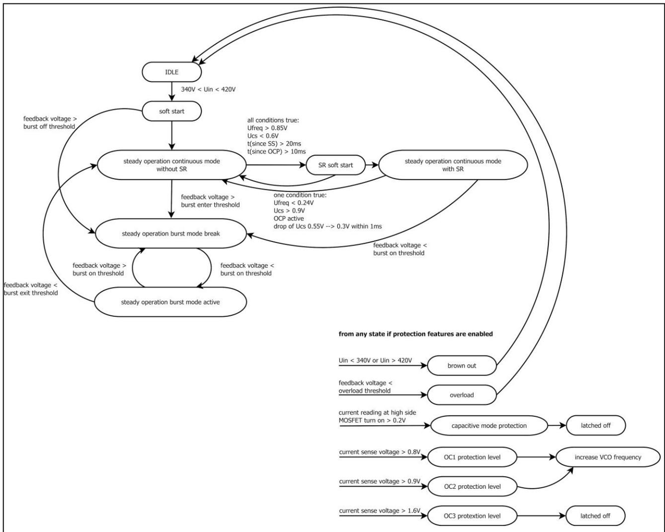
Figure 35 LLC operational state machine implementation using XMC4200
