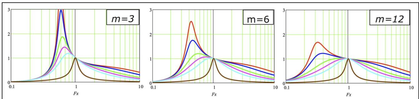
Figure 10 Family of Q curves for m inductance ratios of 3, 6, and 12
