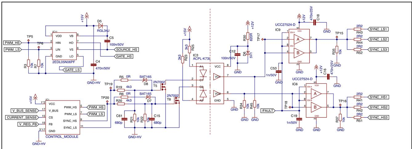
Figure 28 Primary and secondary side driver circuitry
