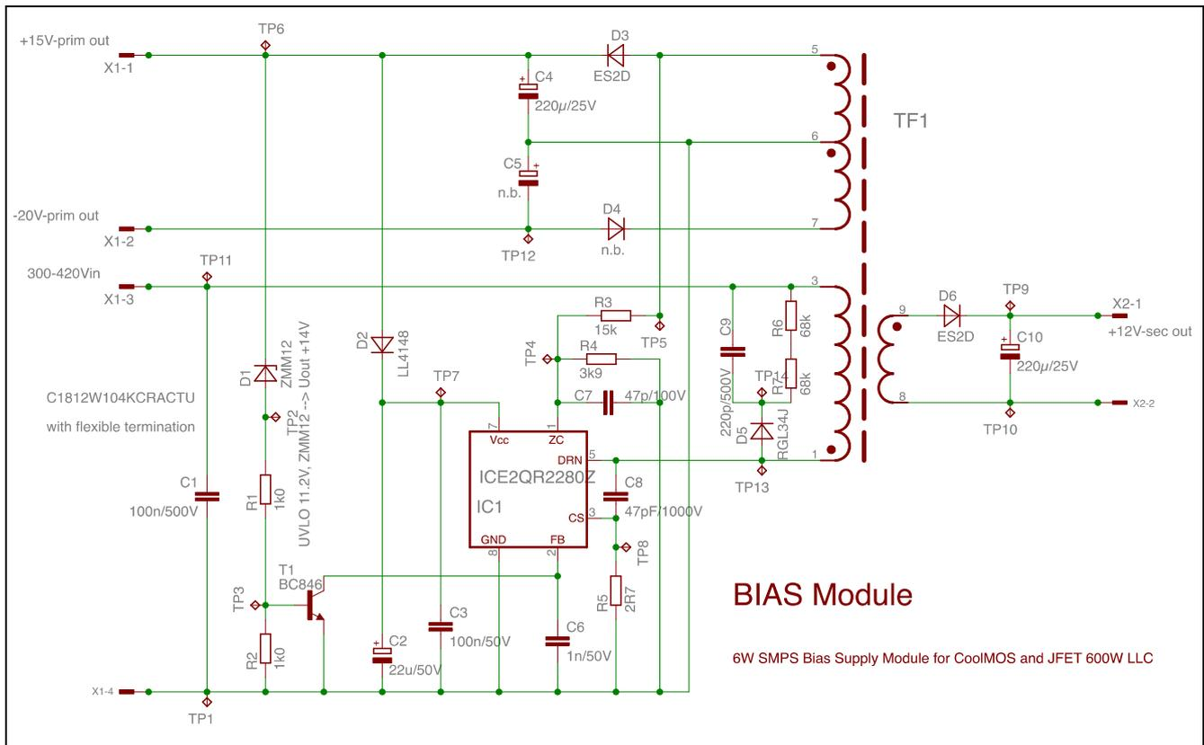
Figure 32 Biasboard schematic
