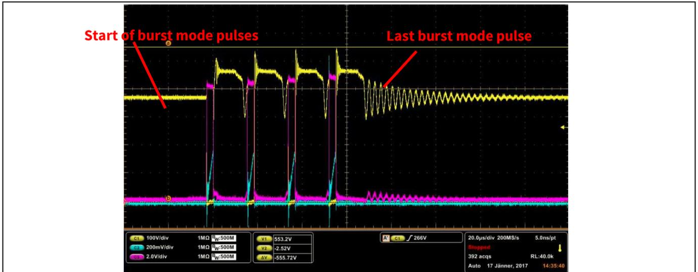
**Figure 20** High line (265 V<sub>AC</sub>), no load. The ICE2QS03G is operating in burst mode to minimize idle power consumption. The burst mode pulse train shown above occurs every 33.8 ms. QR valley switching does not occur during burst mode due to the ICE2QS03G changing operating modes at light load. V<sub>DS</sub> maximum is only 553 V in burst mode operation.
