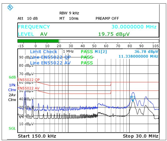
Figure 18 Conductive EMI measurement of the evaluation board at 65 kHz with a resistive load and filter modification (3pin configuration)
