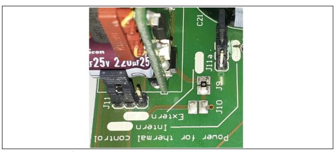
Figure 4 Setting for internal cooling powering
