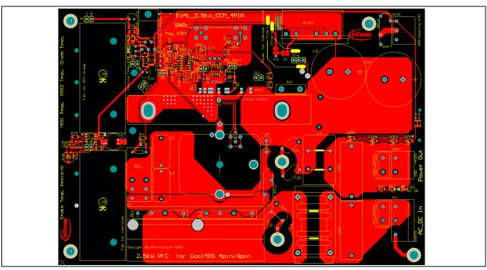
Figure 7 PCB top layer view
