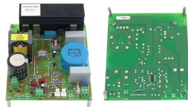
300 W CCM PFC evaluation board for SMPS with high efficiency and high power factor; featuring IPP60R190P6 (CoolMOS™ P6)
