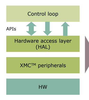
Target: Ensure code reusability and reliability by isolating control loops from HW
