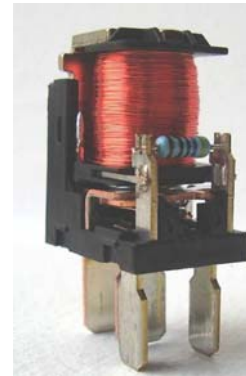
Figure 3 Electrical schematic vs. Picture of Relay with built in parallel resistor
