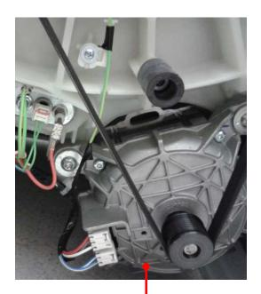
Washing machine PMSM motor
