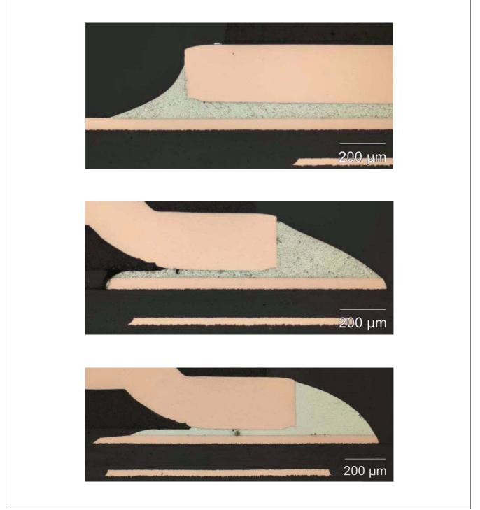
Figure 19 Cross Section Views of Mounted TDSON-8 Packages. The first photo shows a SnPb solder joint of the drain pad. The second and third photos show source/gate solder joints with SnPb, and SnAgCu alloys, respectively.
