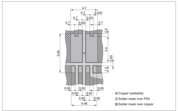
Figure 8 Recommended PCB Pad Design for Dual SuperSO8
