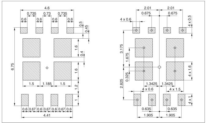
Figure 14 Recommended dimensions of solder paste stencil for Dual SuperSO8 with 50% coverage of drain pad area; alternative dimensioning at the right side
