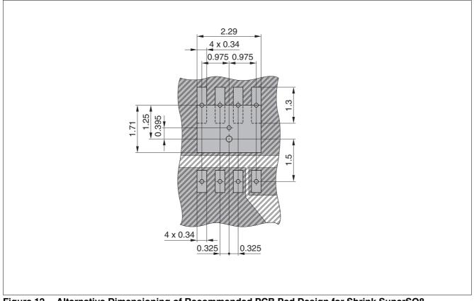
Figure 12 Alternative Dimensioning of Recommended PCB Pad Design for Shrink SuperSO8
