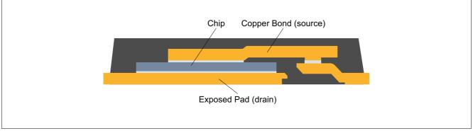
Figure 2Cross Section Showing Construction of Clip Bond
