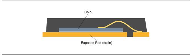
Figure 1 Cross Section Showing Construction of Wire Bond
