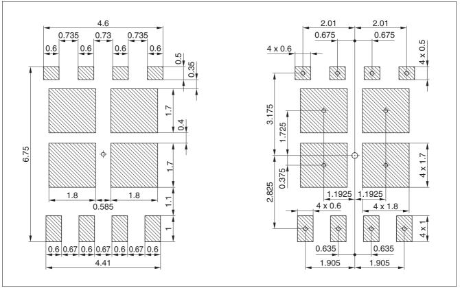
Figure 13 Recommended dimensions of solder paste stencil for SuperSO8 with 55% coverage of drain pad area; alternative dimensioning at the right side
