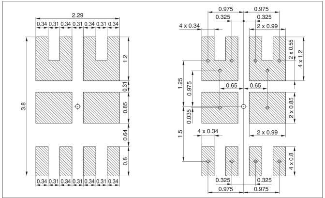
Figure 15 Recommended dimensions of solder paste stencil for Shrink SuperSO8 with 75% coverage of drain pad area; alternative dimensioning at the right side
