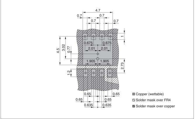
Figure 10 Alternative Dimensioning of Recommended PCB Pad Design for SuperSO8
